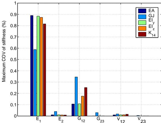
Figure 2: Sensitivity of baseline cross-sectional stiffness to material properties
