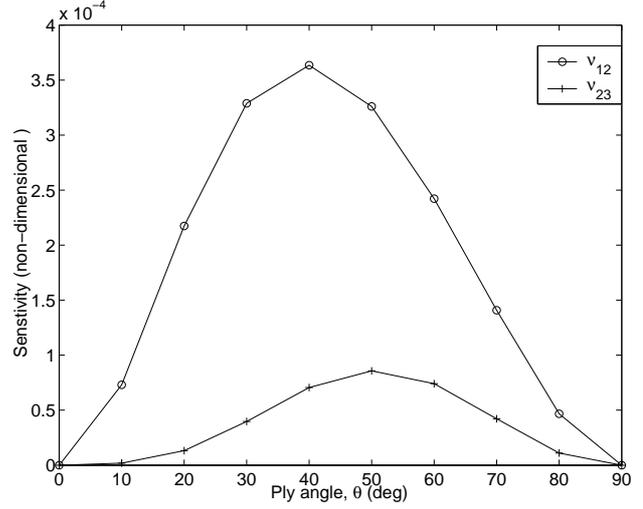
Figure 5: Sensitivity of torsional stiffness to Poisson's ratio
