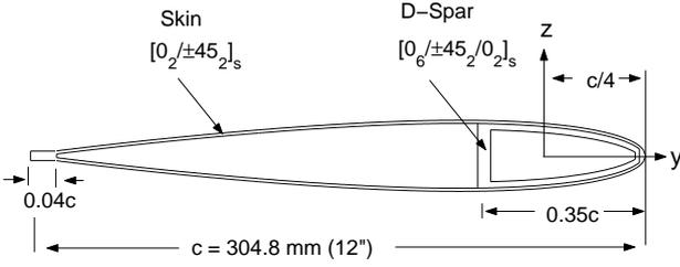
Figure 1: Elastic rotor blade
