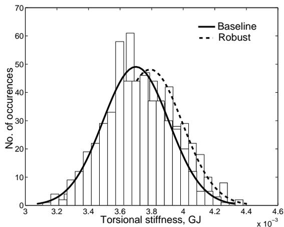
Figure 12: Histograms of torsional stiffness
