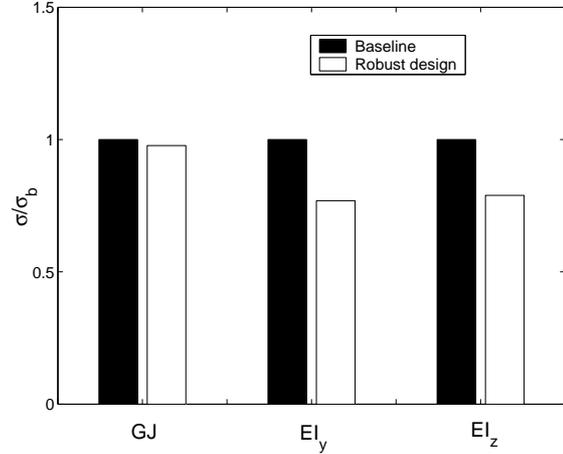
Figure 9: SD of baseline and robust designs, normalized with baseline values
