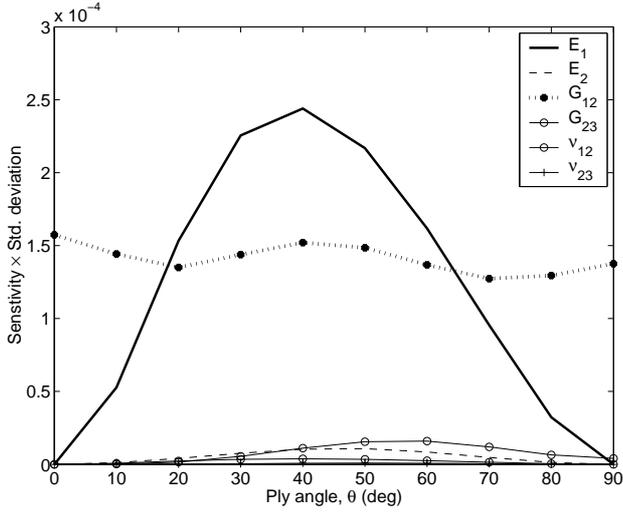
Figure 7: Effect of stacking sequence on SD of torsional stiffness
