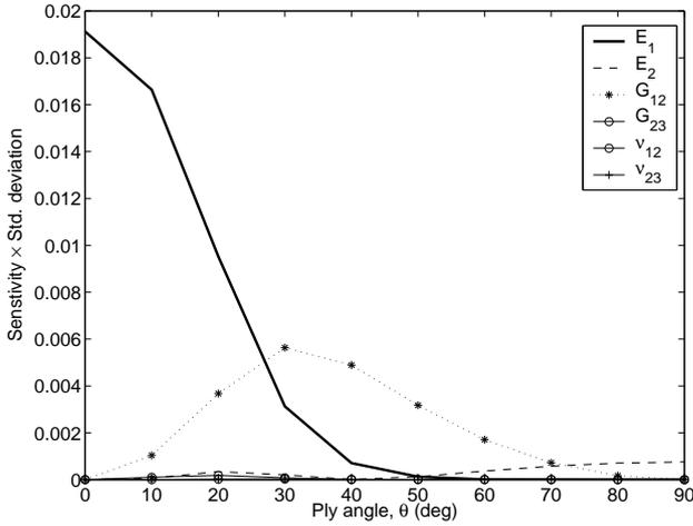
Figure 8: Effect of stacking sequence on SD of lag stiffness
