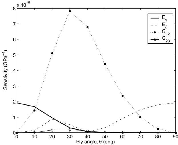
Figure 4: Sensitivity of lag stiffness to elastic moduli
