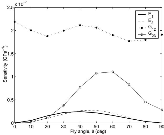
Figure 3: Sensitivity of torsional stiffness to elastic moduli
