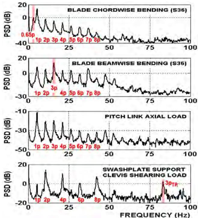
Figure 20: FLMS Spectrum Survey, Roll-Reversal
