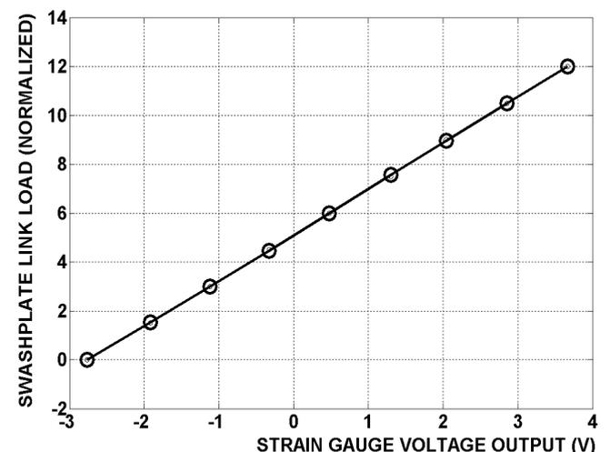
Figure 10: Typical Strain Gauge Calibration Curve
