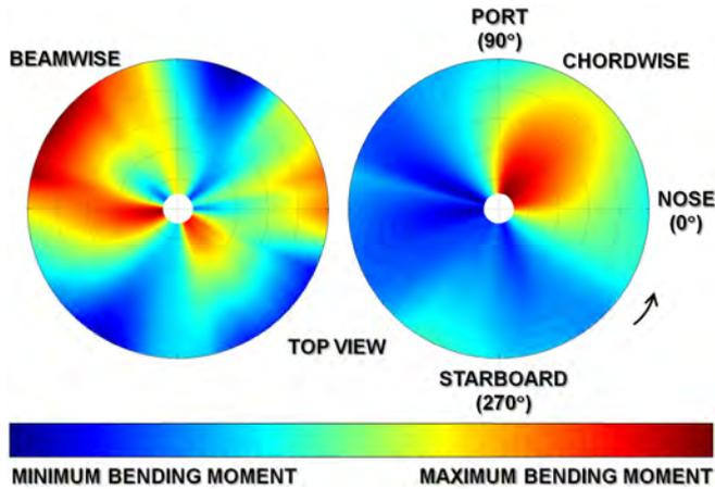
Figure 19: Blade Bending Moments, Roll Reversal
