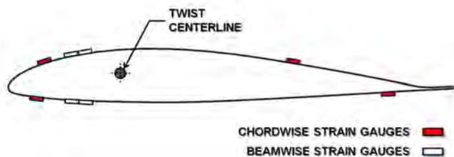
**Figure 5:** Bell 412 Instrumented Blade Section, Station S132
