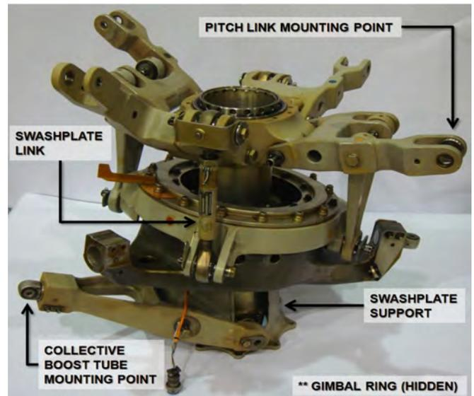
**Figure 7:** Bell 412 Instrumented Swashplate Assembly
