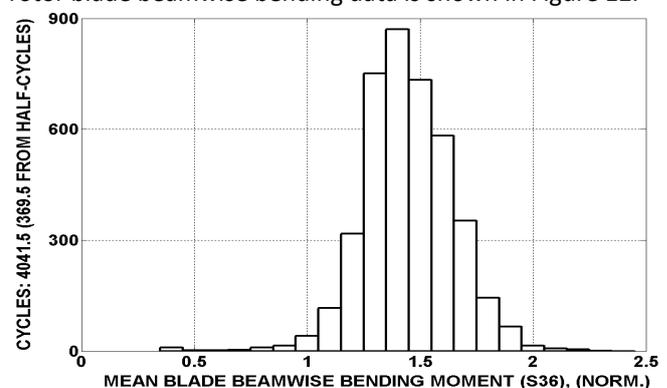
Figure 12: Cycle Histogram, Beamwise Blade Bending Data
