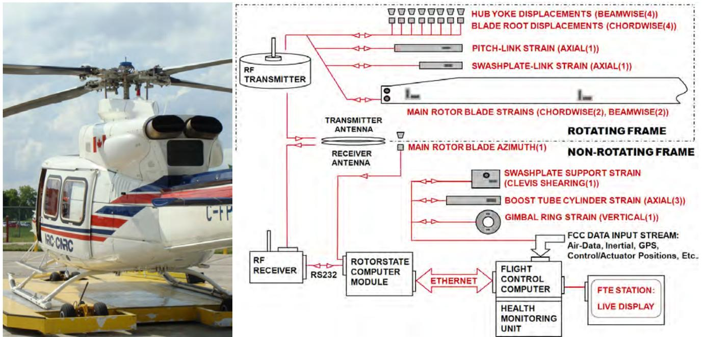
**Figure 3:** Integrated Bell 412 ASRA Flight Loads Measurement Suite (FLMS) Architecture
