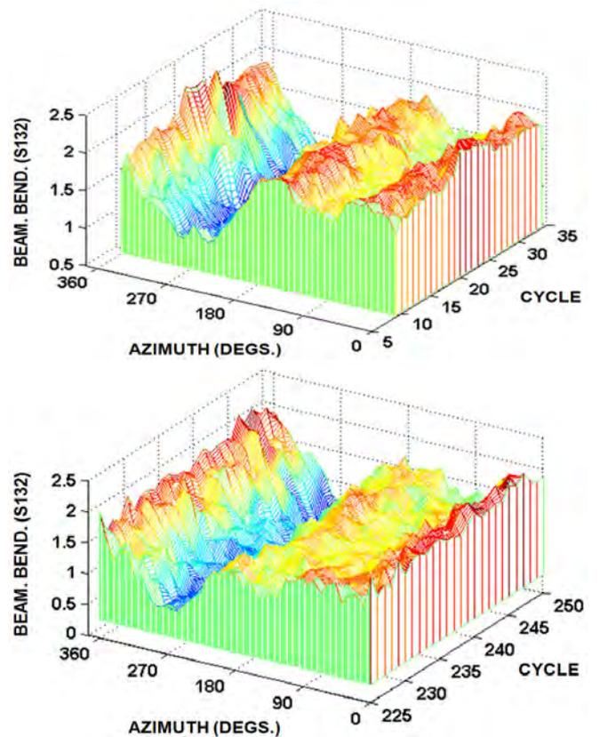
Figure 18: Consistency: Blade Bending in Steady Hover (Top) CW/σ = 0.061, (Bottom) CW/σ = 0.057, (Counter-Clockwise Rotor Revolution: Nose = 0° ; Port-Side = 90°)
