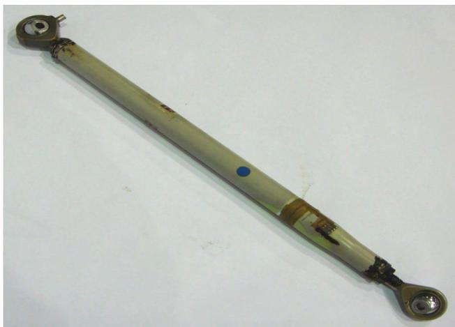
**Figure 6:** Bell 412 Instrumented Main Rotor Pitch Link
