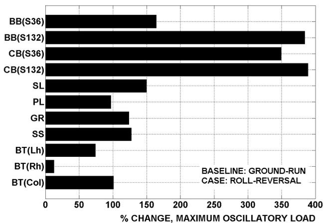
Figure 16: Percent Change in Maximum Oscillatory Loads, Flight Roll Reversal vs. Ground-Run Lateral Cyclic Sweep
