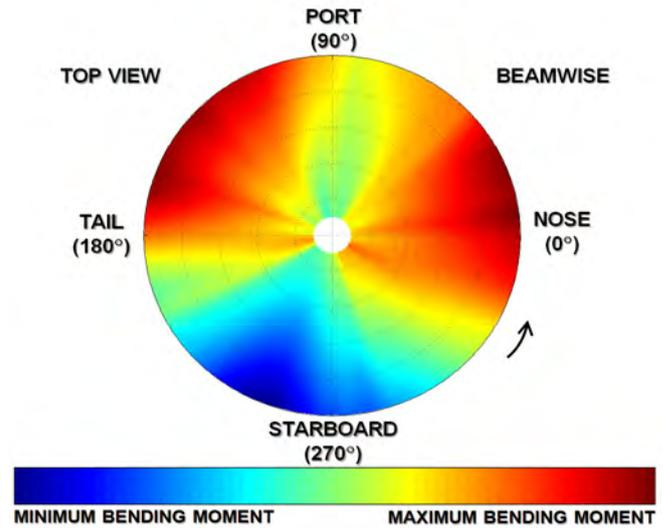
Figure 11: Polar Surface Plot, Beamwise Blade Bending Data
