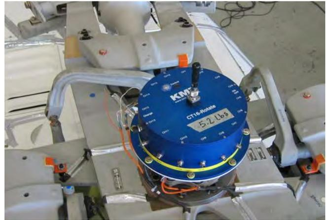
**Figure 2:** Bell 412 ASRA RSMS Hub Mounted Transmitter
