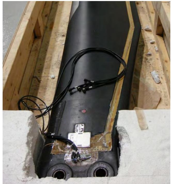
**Figure 4:** Bell 412 Instrumented Main Rotor Blade
