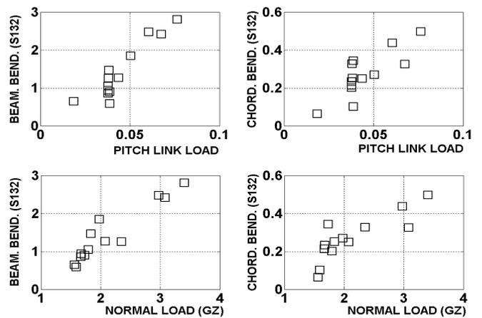
Figure 17: Trending: Blade Bending, Pitch Link Load, and Gz
