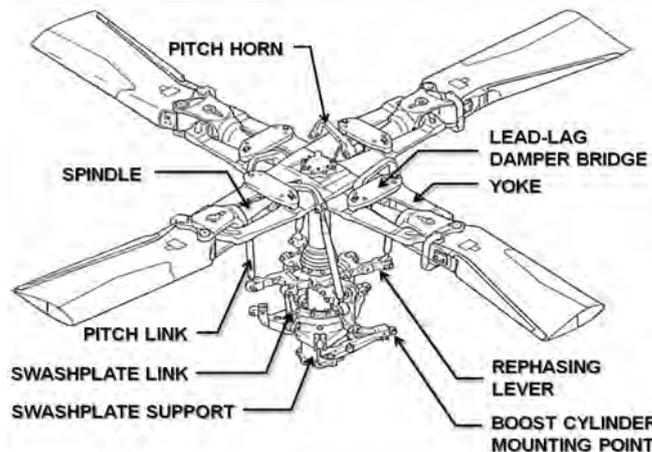
**Figure 1:** NRC-FRL Bell 412 ASRA, Hingeless Rotor Hub, and Rotor System Controls [8].
