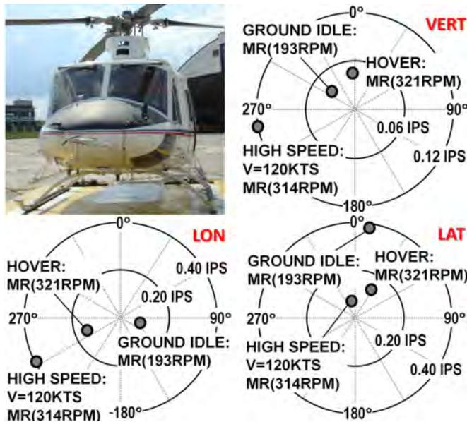
Figure 13: Typical 1/rev RADS™ Systems Vibration Survey
