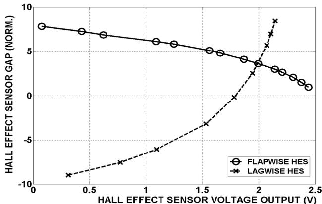
Figure 8: Typical Hall Effect Sensor Calibration Curves
