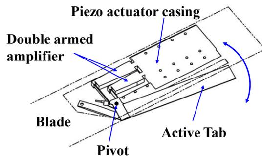
Figure9: Drive mechanism of Active Tab
