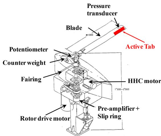
Figure 3: One-bladed rotor system with Active Tab
