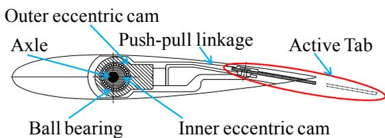
Figure6: Drive mechanism : servo motor with eccentric cam
