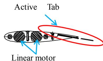
Figure 7: Drive mechanism : linear motor with bell crank
