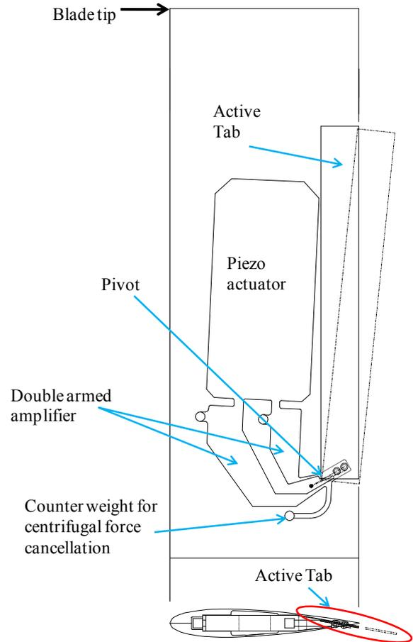
Figure 5: Drive mechanism : piezo actuator with elastic hinges
