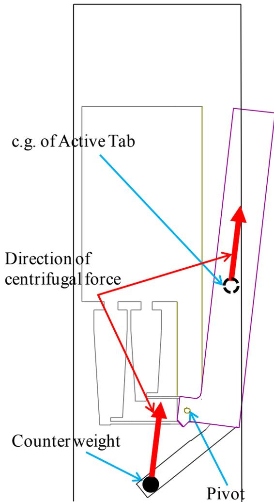
Figure10: Counter weight installation
