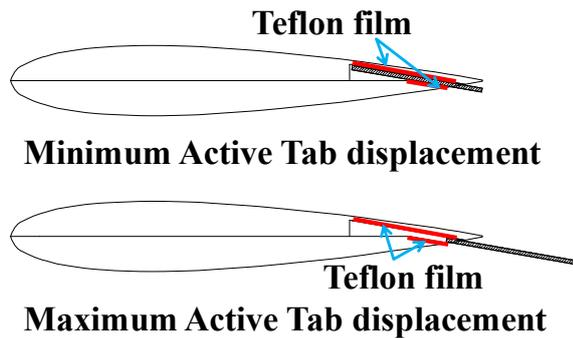
Figure12: Friction reduction measure for Active Tab operation
