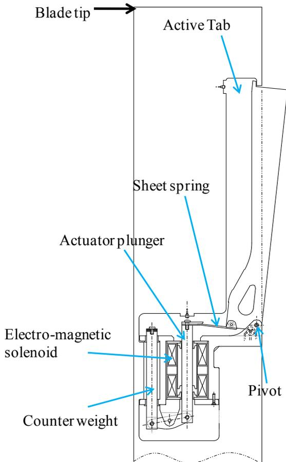
Figure 8: Drive mechanism : electro-magnetic solenoid with sheet spring
