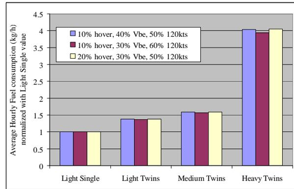
**Figure 8:** Impact of Time Distribution in an Average Mission Spectrum
