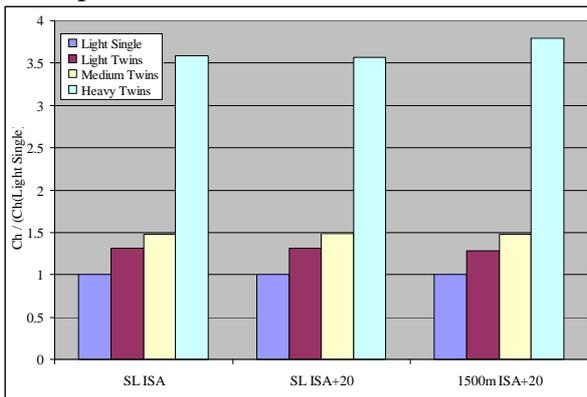
**Figure 6:** Relative Hourly Fuel Consumption of Four Example Helicopters, at their MTOW at 120kts, for Different Atmospheric Conditions, normalized with Light Single values
