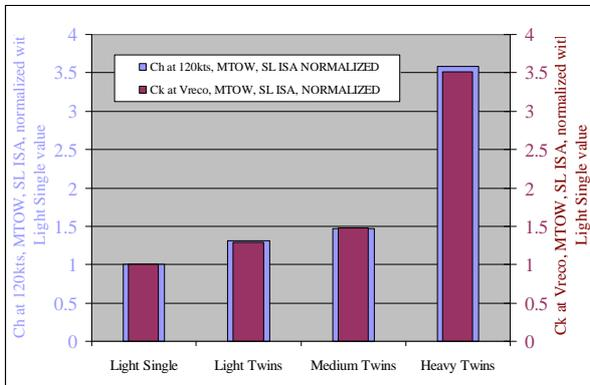
**Figure 7:** Comparison of Hourly Fuel Consumption at 120kts and Kilometric Fuel Consumption at Vreco
