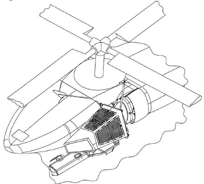
Fig. 1: IBF for Sikorsky UH-60 Blackhawk, according to U.S. Patent 7192462 [1].
