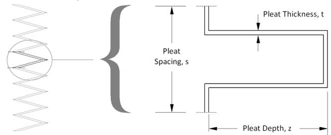
Fig. 4: Idealised Pleat Configuration for CFD Analysis.
