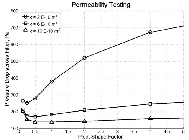
Fig. 9: Effect of Filter Permeability on Pressure Drop.
