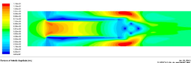
Fig. 12: Velocity Magnitude distribution across pleat of Shape Factor 0.5 and pleat spacing 100 mm (pleat depth: 200 mm).
