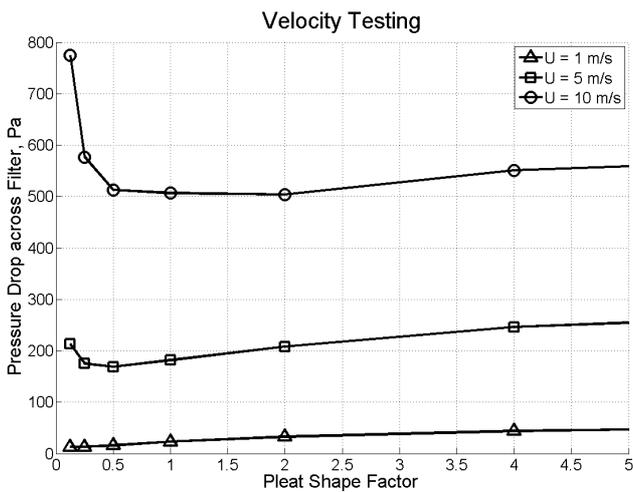
Fig. 7: Effect of Approach Velocity on Pressure Drop.
