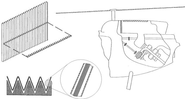
Fig. 2: Example of pleated filter for IBF application, according to U.S. Patent 6595742 [4].
