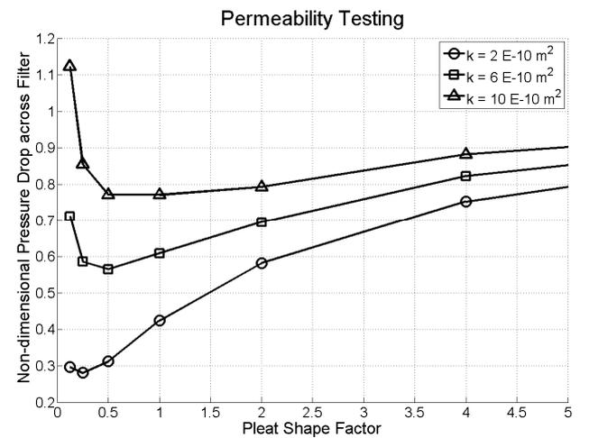
Fig. 10: Effect of Filter Permeability on Non-dimensionalised Pressure Drop.
