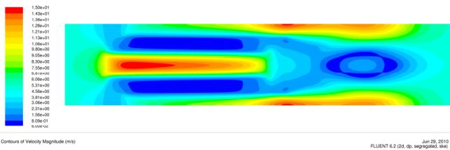
Fig. 11: Velocity Magnitude distribution across pleat of Shape Factor 0.5 and pleat spacing 10 mm (pleat depth: 20 mm).
