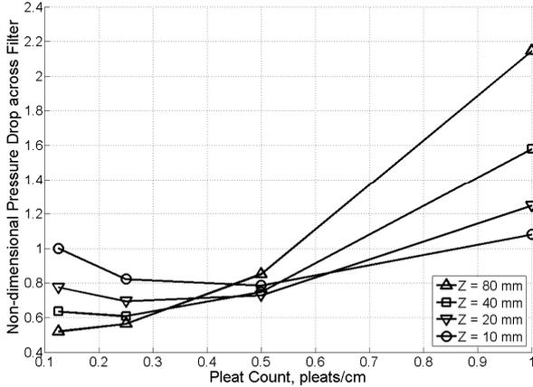
Fig. 13: Pressure drop across a pleated filter as a function of pleat count for four pleat depths.
