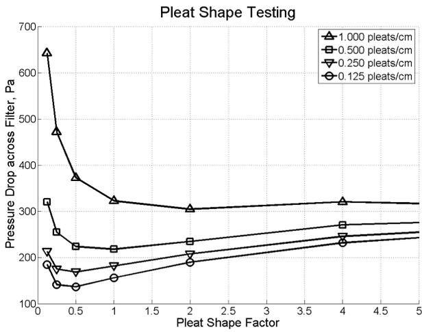
Fig. 5: Effect of Pleat Shape Factor and Pleat Count on Pressure Drop.
