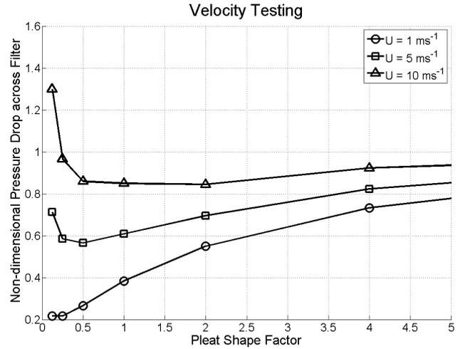
Fig. 8: Effect of Approach Velocity on Non-dimensionalised Pressure Drop.
