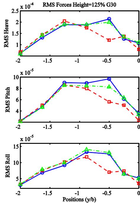
Figure 13: RMS Forces and Moments for G30 Baseline SRF (—○—), SRF with 30° angled flap (—■—) and saw-tooth flap (·-△-·)
