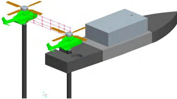
Figure 6: AirDyn test-point location grid with AirDyn pictured at port side approach position and spot hover location
