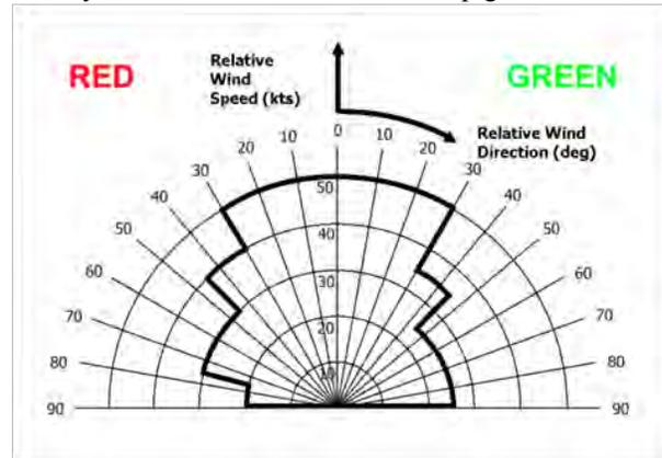
Figure 2: Ship-Helicopter Operating Limits (SHOL) diagram for Sea-Hawk (SH-60B) helicopter operating to a Simple Frigate Shape (SFS2) derived from flight simulation at the UoL
