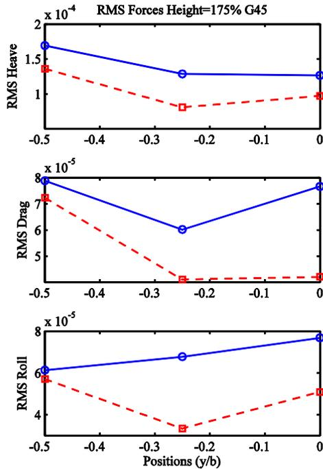
Figure 11: RMS Forces and Moments for G45 Baseline SRF (—○—) and SRF with Side Flap modification (-■-)
