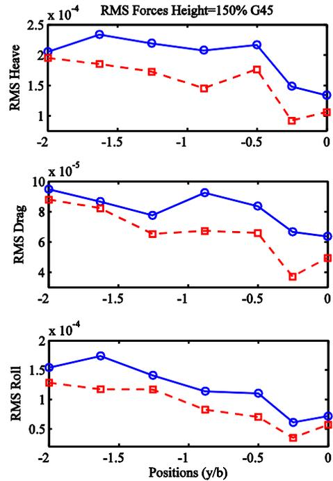
Figure 10: RMS Forces and Moments for G45 Baseline SRF (—○—) and SRF with Side Flap modification (---□---)
