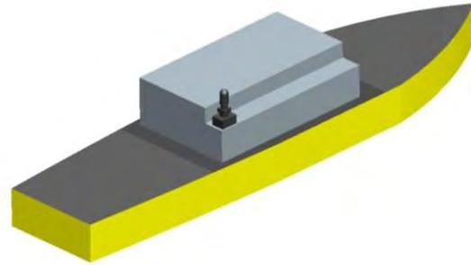
Figure 15: SRF with hangar notch and Phalanx Close-In-Weapons-System (CIWS)
