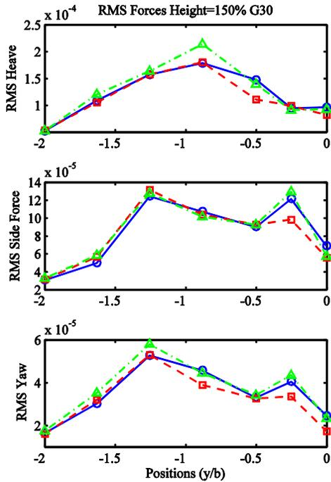
Figure 14: RMS Forces and Moments for G30 Baseline SRF (—○—), SRF with 30° angled flap (—■—) and saw-tooth flap (—△—)
