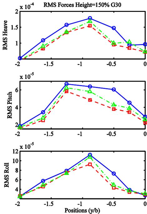
Figure 17: RMS Forces and Moments for G45 Baseline SRF (—○—), SRF with Hangar Notch without (---□---) and with Phalanx CIWS (-·-△-·-)
