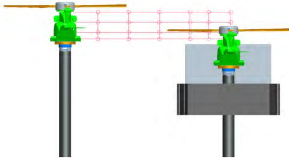
Figure 7: Lateral traverse rotor heights (110%, 125%, 150% & 175% HH)
