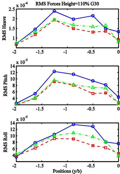
Figure 16: RMS Forces and Moments for G45 Baseline SRF (—○—), SRF with Hangar Notch without (---□---) and with Phalanx CIWS (-·-△-·-)
