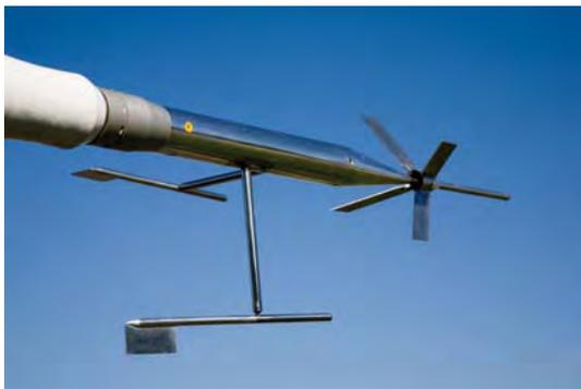
Figure 2: FHS noseboom with airflow and pitot sensors
