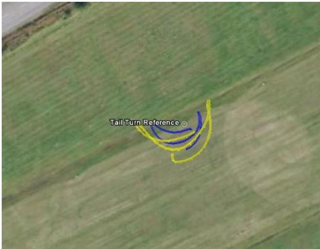
Figure 4: Bell 206 position data for tail-turns done with NVG A (yellow) and NVG B (blue).
