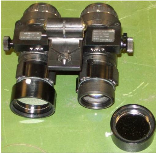
Figure 2: NVG with neutral density filter on right-eye tube; left-eye tube filter holder shown in lower right corner
