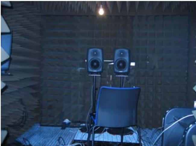
Fig. 5: Acoustic simulator in anechoic chamber
