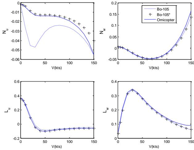
**Figure 14. Coupling derivatives for longitudinal and lateral motions**
