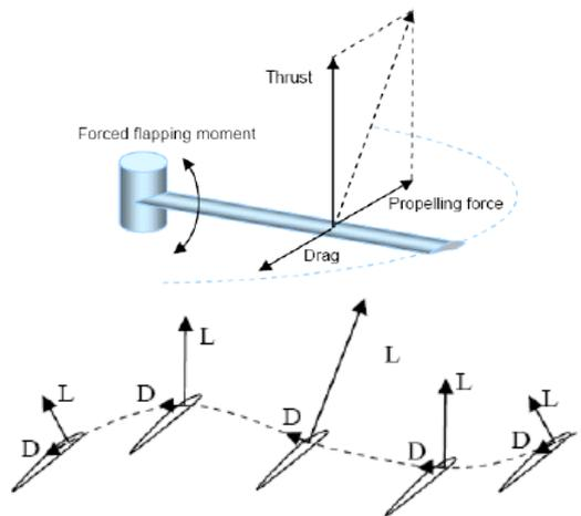
**Figure 2. Lift and drag forces acting on an Ornicopter blade during one revolution when a constant pitch angle is applied [Ref. 10]**
