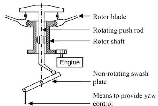
**Figure 4. Principle of a flap forcing mechanism using a push-pull rod and swashplate [Ref. 4]**
