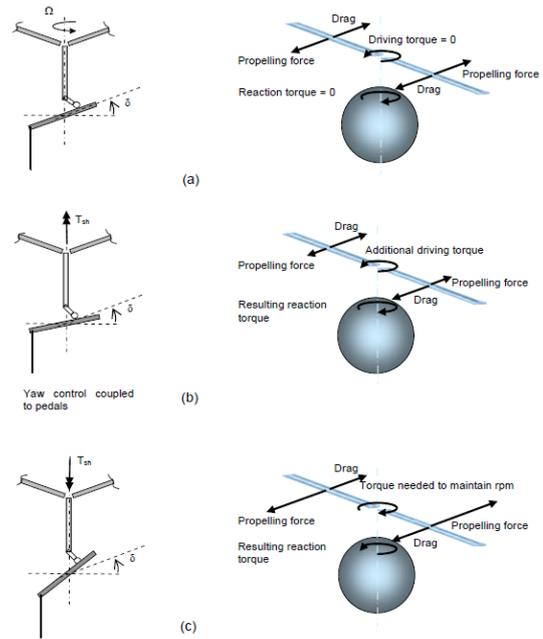
**Figure 6. Schematic representation of yaw control by introducing a reaction torque**
