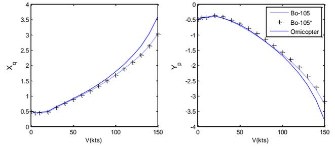
**Figure 15.  $X_q$  and  $Y_p$  as a function of flight speed**
