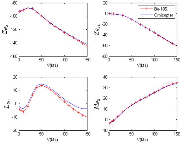
**Figure 18. First set of control derivatives a function of flight speed**
