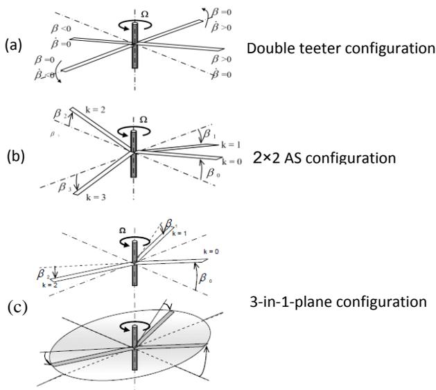
**Figure 1. Three Ornicopter configurations**
