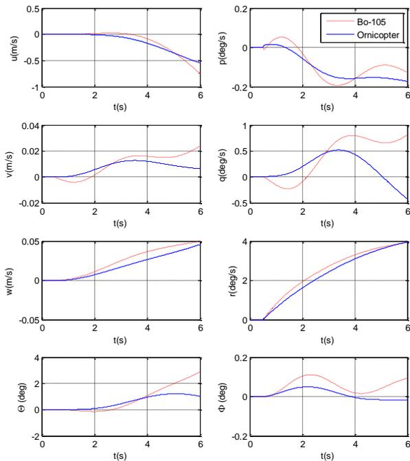
Figure 21. Response to yaw step control input
