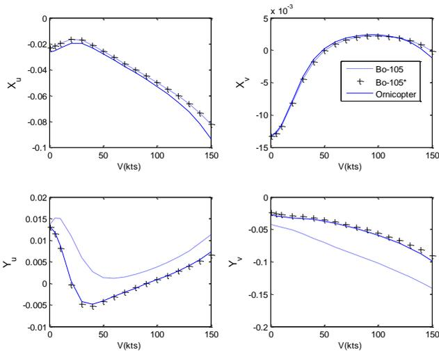
**Figure 10. Direct and coupling force derivatives as a function of flight velocity**
