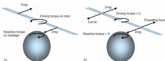
**Figure 3. Forces and moments acting on a conventional helicopter (a) and the Ornicopter (b) [Ref. 10]**
