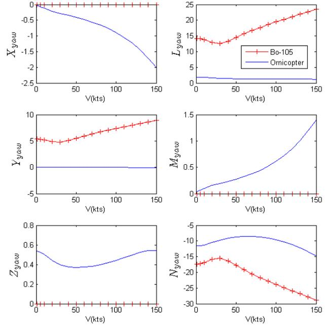
**Figure 20. Yaw control derivatives a function of flight speed**
