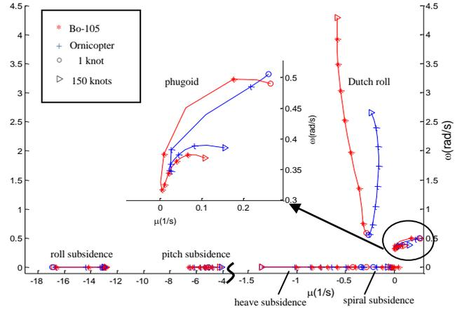
**Figure 8. Loci of Ornicopter and Bo-105 eigenvalues as a function of forward speed**
