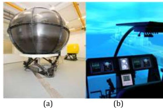
Figure 2: The University of Liverpool's HELIFLIGHT-R motion base flight simulator outside (a) and inside (b) view.
