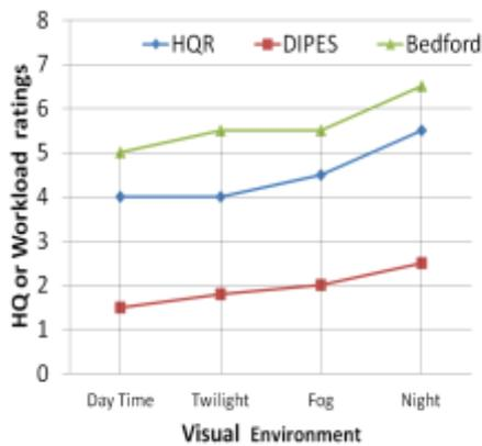
Figure 6: Pilot workload and handling quality ratings in GVE and DVEs, green 45 airwake at wind speed of 30 kts, sea state 5.
