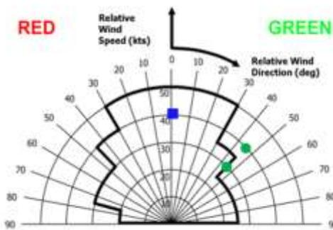
Figure 1: Ship-Helicopter Operating Limits (SHOL) diagram obtained in the Liverpool flight simulator [4]. The square and circular marks indicate the test points in this study.
