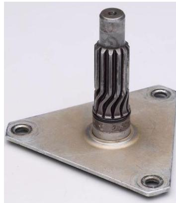
Fig.6 Deformed spline
