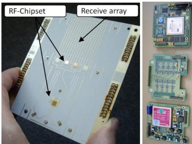
Fig. 5. Fabricated RF-frontend with RF-chipset, an antenna-array (left) and PCBs for complete sensor (right).
