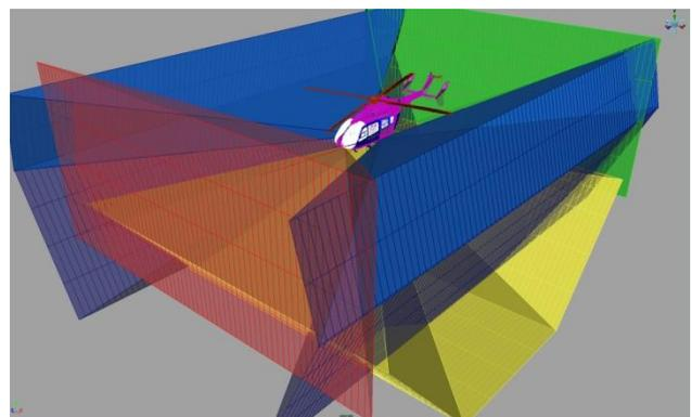
Fig. 4. Distributed sensor arrangement and sensor field of views on helicopter.
