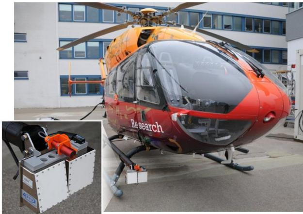
Fig. 12. SITA mounted on EC145 research test bed.
