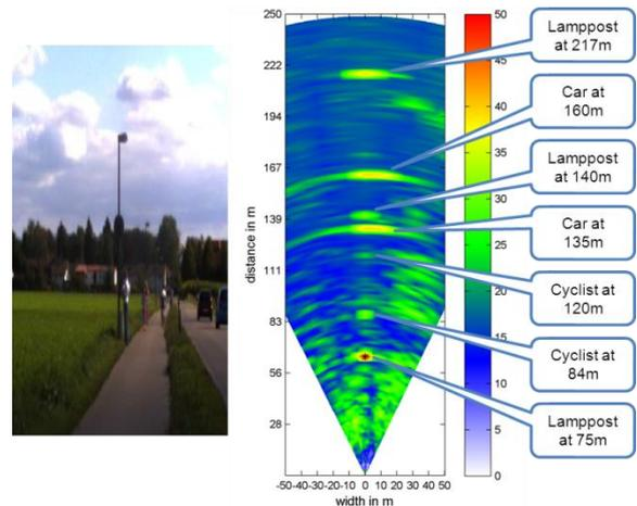
Fig. 10. Measured 2D radar plot of several relevant vertical obstacles with corresponding camera image.
