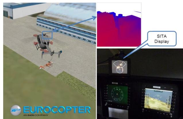
Fig. 16. Sensor Installation in EVE (left), an example of the range image input (upper right), the additional SITA HMI display (lower right).
