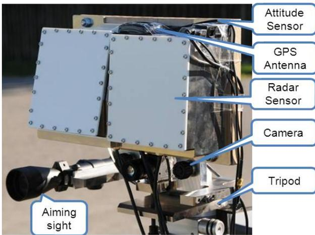
Fig. 8. Setup of the radar prototype for static field tests.
