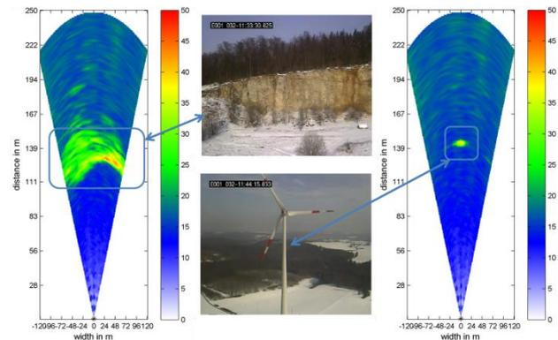
Fig. 13. Flight test 2D radar plots showing the raw reflected intensities in dB of a rock face at ~120m distance (left) and a wind turbine at ~140m distance (right).
