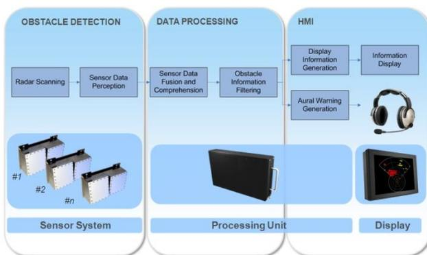
Fig. 3. Functional breakdown and system design for stand-alone (i.e. retrofitable) solution.
