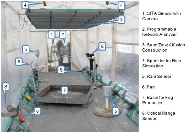
Fig. 14. Test setup for measurement of atmospheric attenuation.
