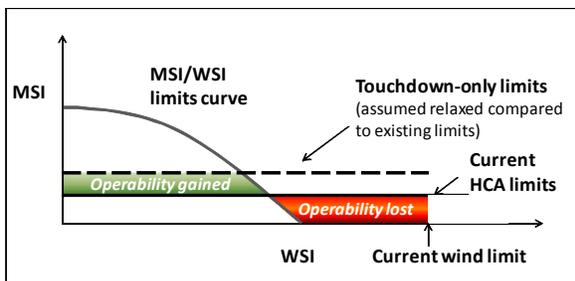
Figure 7: An illustration of the effect of new MSI/WSI limits on operability
