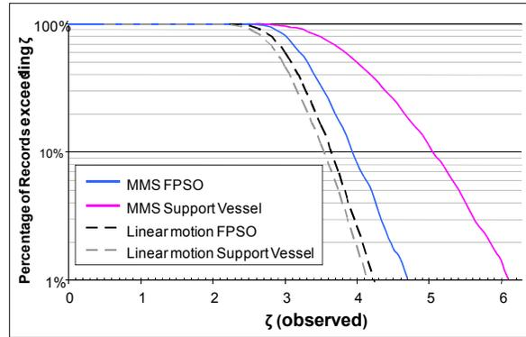
Figure 2: MMS distributions of  $\zeta$  for two vessel types, compared to those for linear motions.
