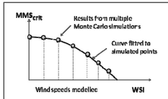
Figure 5: Building the limits curve using Monte Carlo simulations.
