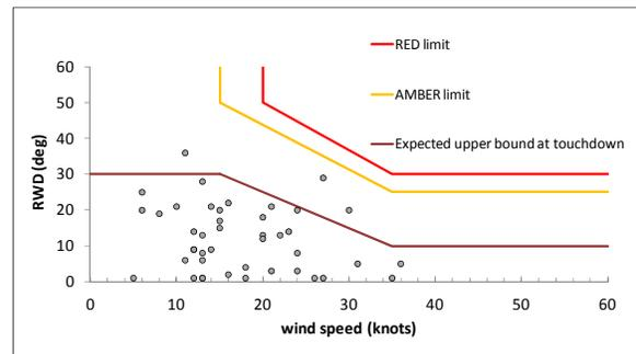
Figure 9: A comparison of GPIII trials data (RWD recorded at touchdown) with the expected upper bound at touchdown and the preliminary RWD limits.
