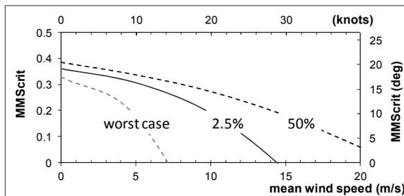
Figure 6: Limits curves calculated for various probabilities.
