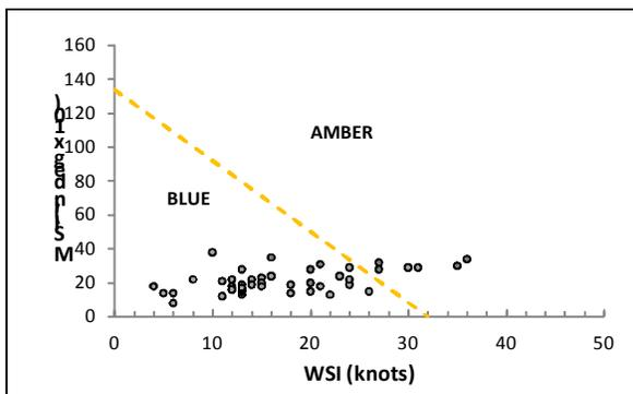
Figure 8: A comparison of GPIII trials data (MSI/WSI recorded just before touchdown) with a preliminary MSI/WSI limits curve.
