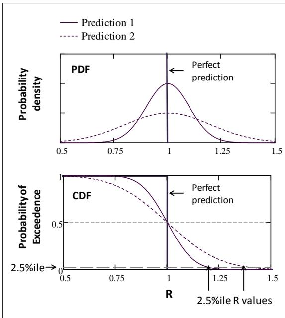
Figure 3: Using ratio R to evaluate forward prediction methods (Prediction 1 is better than 2).
