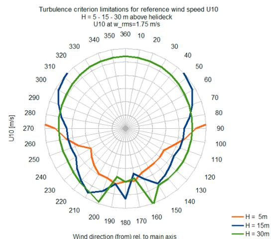
**Figure 2: Turbulence limitations graph**
