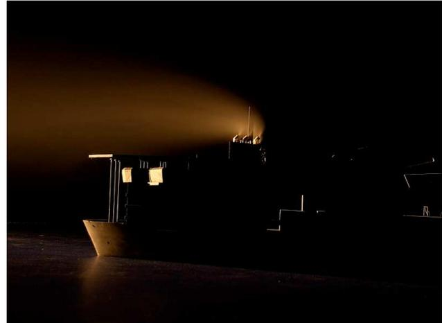
**Figure 1: Exhaust flow visualisation over helideck**
