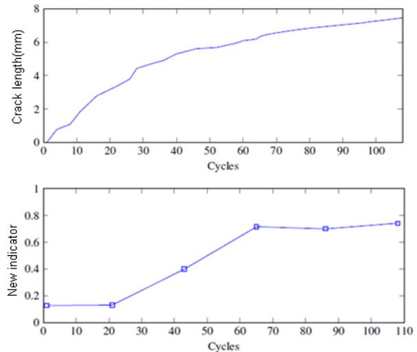
Figure 11: The first graph gives the crack length vs the number of stress cycles and the second graph shows the new indicator vs the number of stress cycles.
