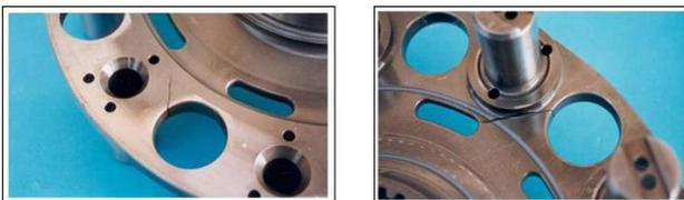
Figure 9: Crack view on each side of the planet carrier
