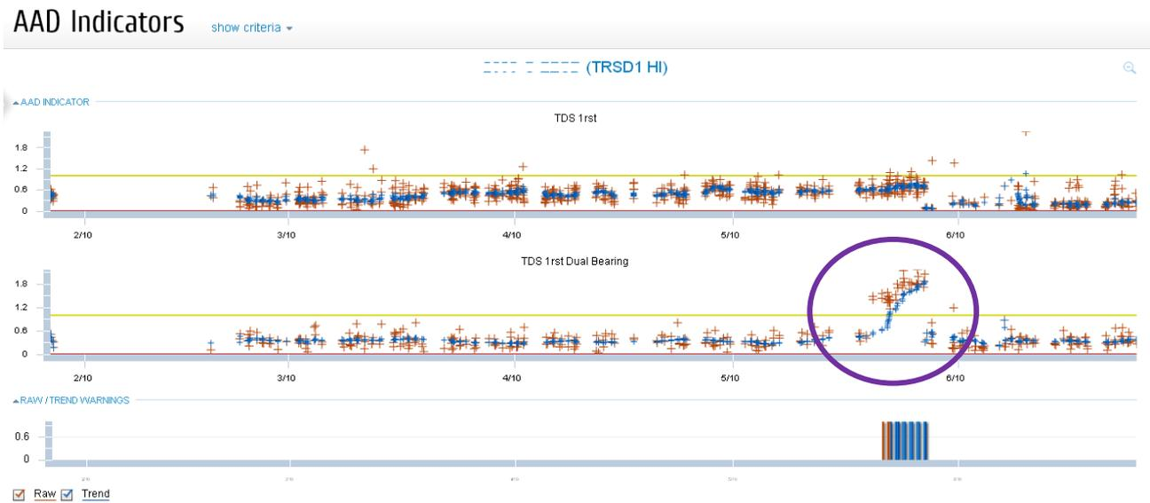
Figure 4: Screenshot of a bearing defect on AAD indicators on WebHUMS (trend visible in the circle)
