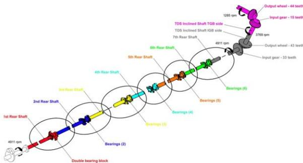
Figure 5: Tail transmission of EC225 (monitored zones during the CSI in the circles)
