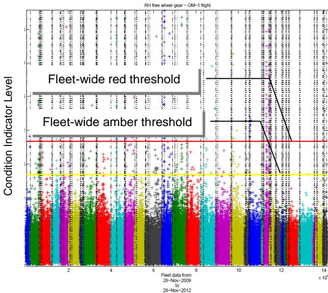
Figure 7 – Fleet-wide threshold based on Gamma distribution shown in a condition indicator series
