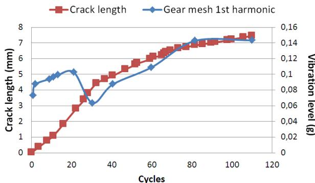
Figure 10: Former condition indicator level vs crack length
