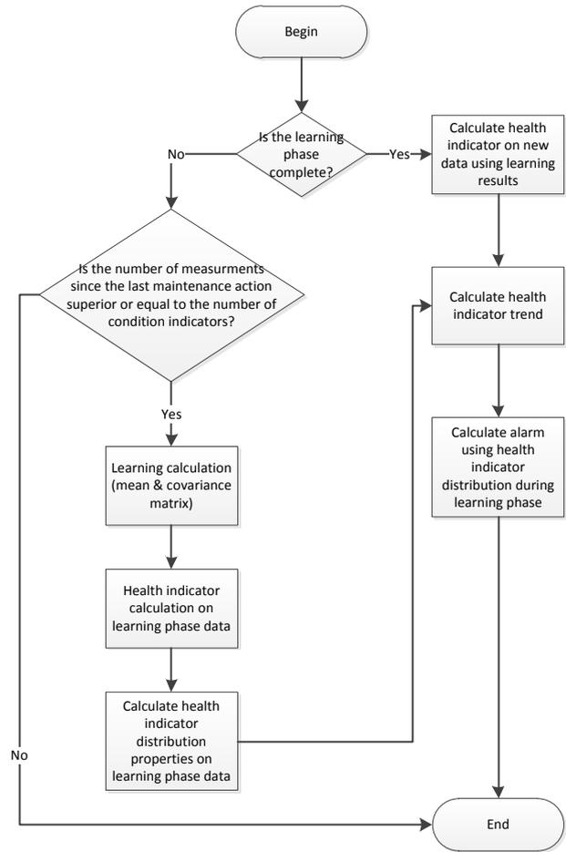
Figure 2: Anomaly detection process
