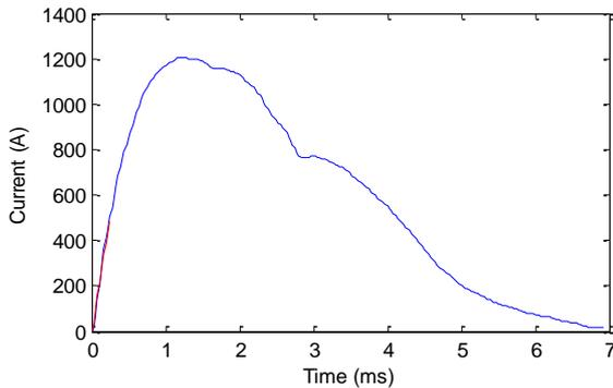
Figure 8: Measured current output from pulse network. Blue indicates measurement from the Rogowski coil, red is from the Pearson 110A current transformer.
