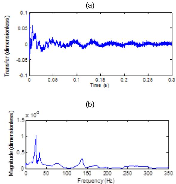
Figure 11: Lift transfer function in (a) time domain and (b) frequency domain.
