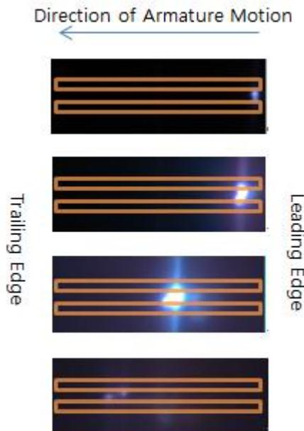
Figure 5: Progression of the plasma armature, from top to bottom, at 0.156 ms, 0.921 ms, 3.146 ms, 5.056 ms referenced from the initial formation of the armature.
