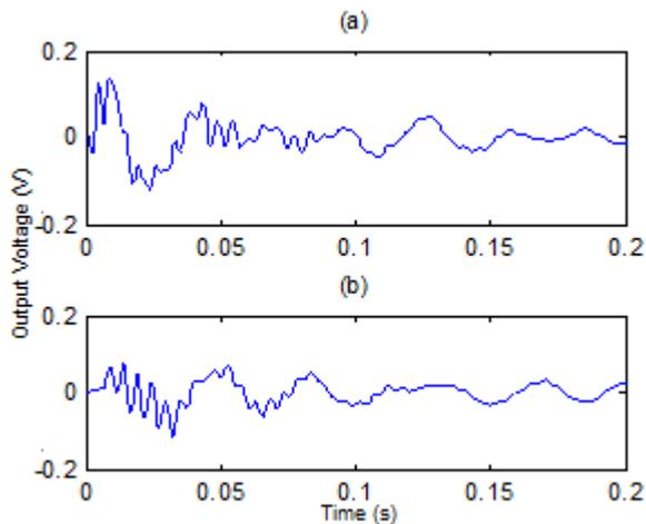
Figure 13: Synchronously averaged lift load cell response from (a) right end of airfoil, (b) left end of airfoil.
