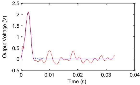
Figure 12: Comparison of actual forcing (shown in blue) and deconvoluted forcing (shown in red) in time domain.
