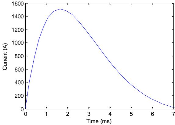
Figure 4: Simulated theoretical response of RailPac pulse current with constant resistance assumption.
