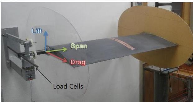
Figure 2: S5010 Test Article with embedded RailPAC system as viewed from the trailing edge. Load cells are mounted on both sides of the airfoil.
