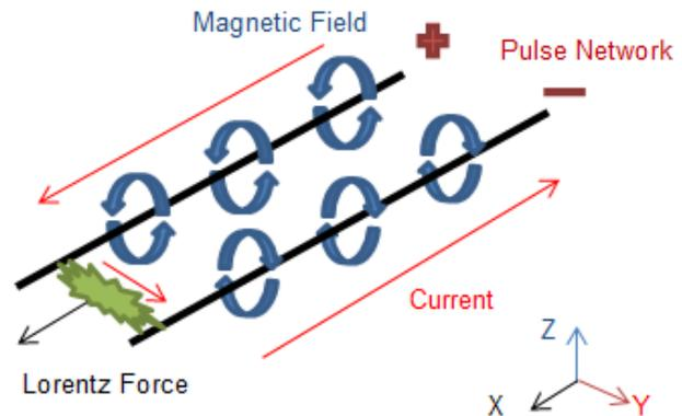
Figure 1: Schematic of the RailPac system.
