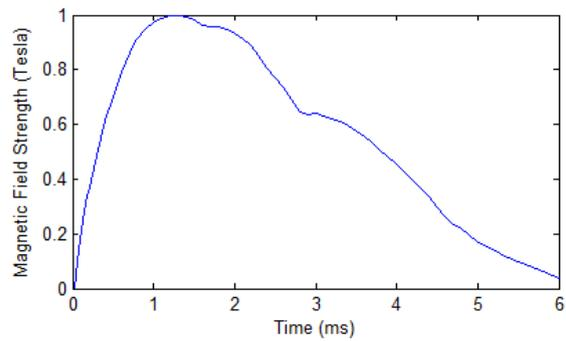
Figure 9: Induced magnetic field strength at the armature position.
