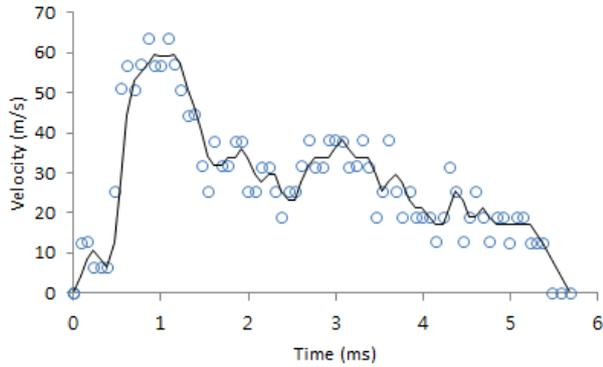
Figure 7: Flow velocity in time domain. Blue scatter plot represents velocity obtained from differentiation. Black line is three-point moving average to emphasize the mean velocity profile.
