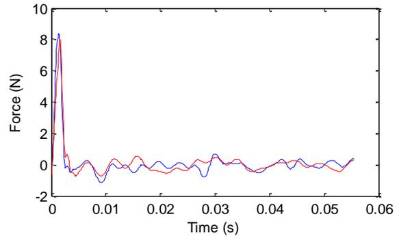
Figure 14: Deconvoluted lift forcing from left end of airfoil in blue and right end of airfoil in red.
