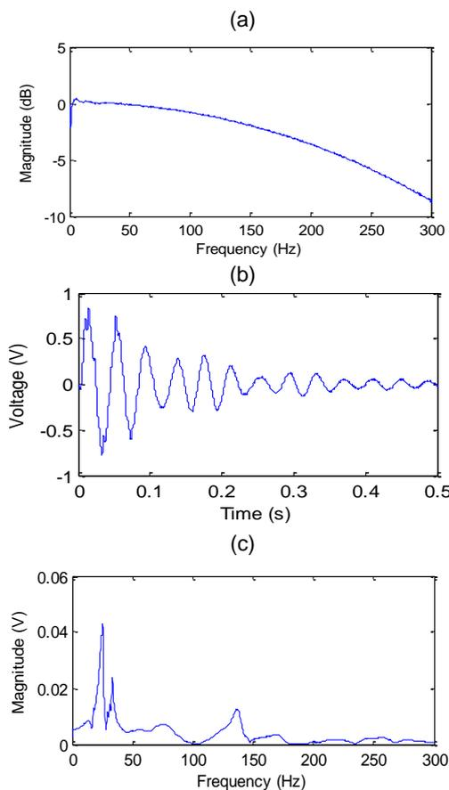
Figure 10: (a) Impulse hammer signal in frequency domain, (b) Lift load cell response in time domain and in (c) frequency domain.
