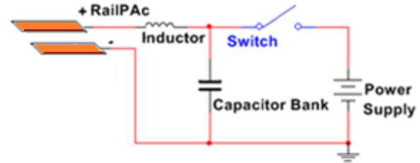
Figure 3: Circuit Diagram of Pulse Network
