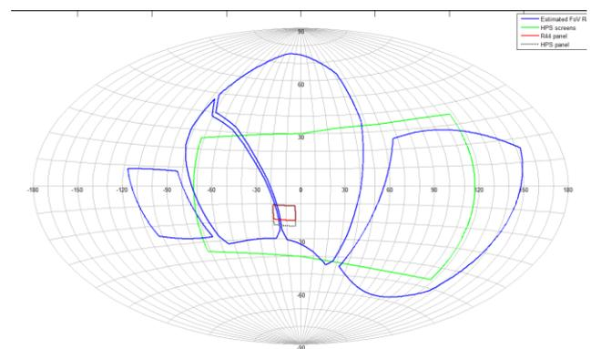
**Figure 1 Optical field-of-view from the pilot’s eye reference point in the HPS, with the new 19” instrument panel, relative to the R44 helicopter.**
