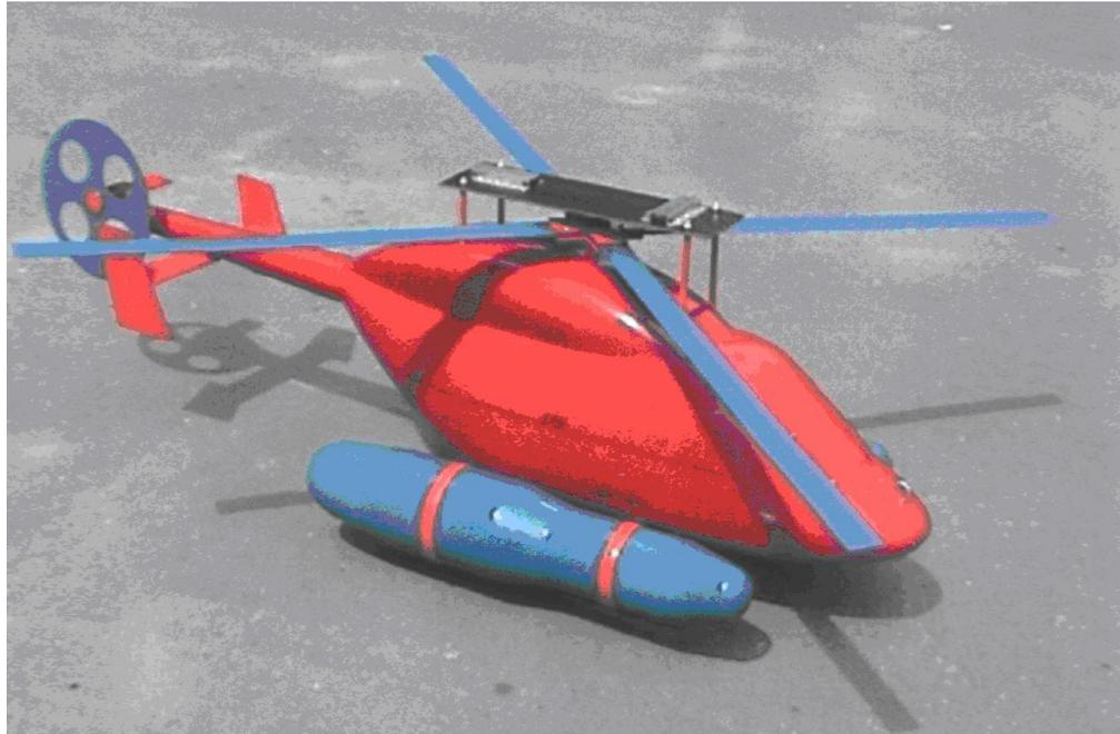
Figure 2 Dynamically similar model of ANSAT helicopter
