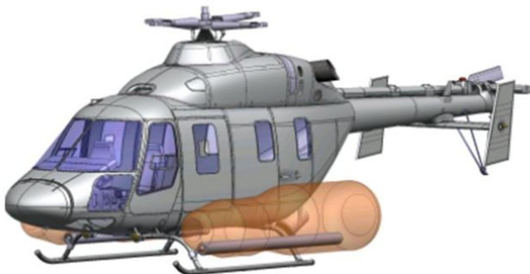
Figure 1 The appearance of ANSAT helicopter with installed EFS
