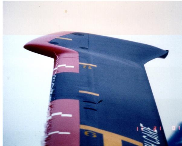
Figure 4. Ice accretion on an EH101 BERP rotor blade.
