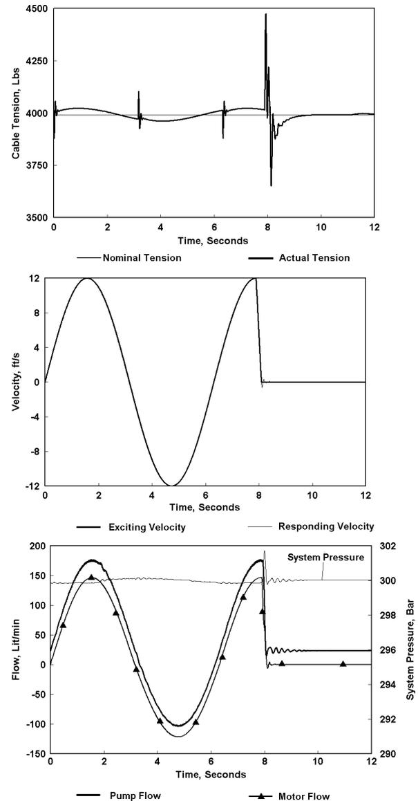
Figure 9 Simulation results of helicopter landing bounce.
