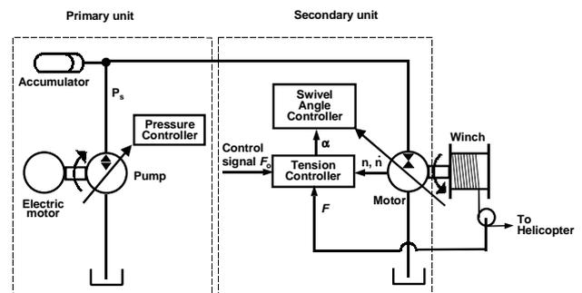
Figure 5 Block diagram of proposed RA cable system.
