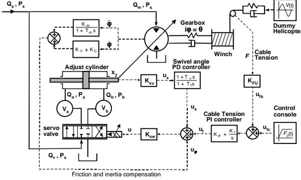
Figure 7 Control block diagram of secondary unit.
