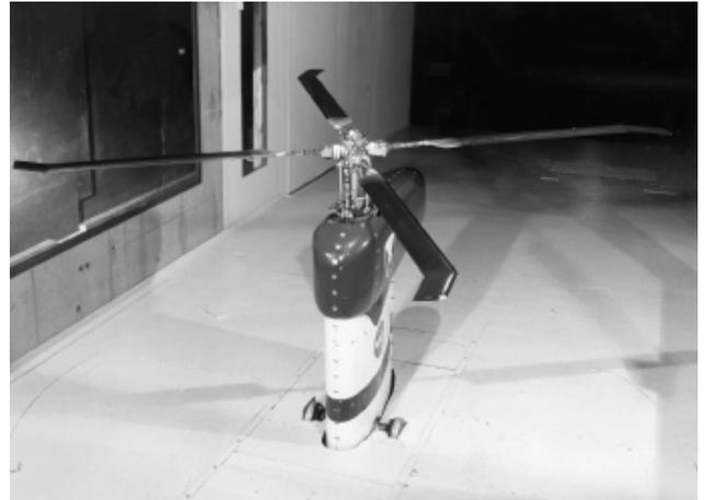
**Fig. 2** Swept-tip rotor on RTR test stand in the Army/NASA 7- by 10-Foot Wind Tunnel.
