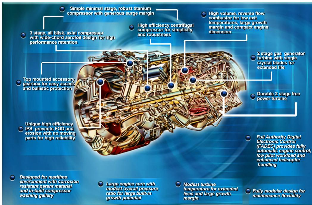
Fig 1 RTM322 Design Features
