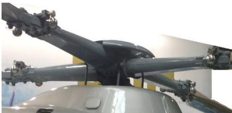
Figure 1: Kazan Helicopter Ansat (above)<sup>1</sup> and main rotor with pendulum absorber (below)<sup>2</sup>
