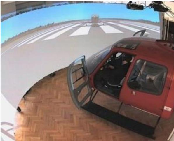
Fig. 1. A flight simulator with the screen and the helicopter cabin
