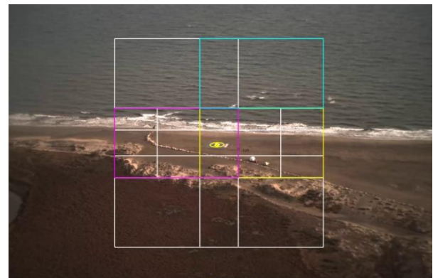
Fig 4: The multi-resolution approach. The input image is divided into many overlapping sub-images.
