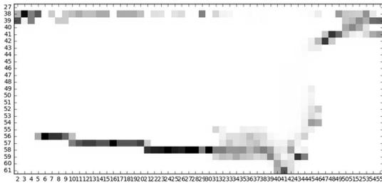
Figure 3: Co-occurrence matrix for all data produced by the aircraft A in a time window of 6h. The oil pressure states are on the X axis and the oil temperature states are represented on the Y axis.
