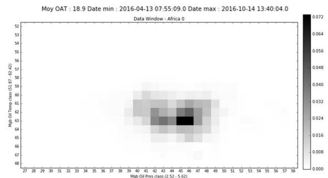
Figure 8: Co-occurrence matrix for data produced by the aircraft A in 212 hours of stabilized flight in Africa.
