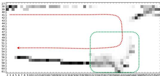
Figure 4: Different phases of flight on the co-occurrence matrix from figure 3. The red arrow sketches the different flight status, whereas the green shape gives the stabilized flight status.
