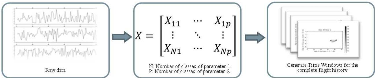
Figure 2: Methodology to build a co-occurrence matrix between states of oil temperature and pressure.
