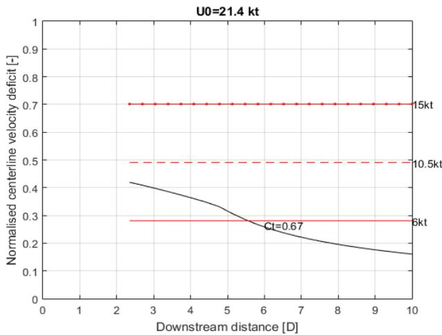
Figure 5 Normalized velocity deficient for  $U_0=11\text{m/s}$  and  $C_t=0.67$ .
