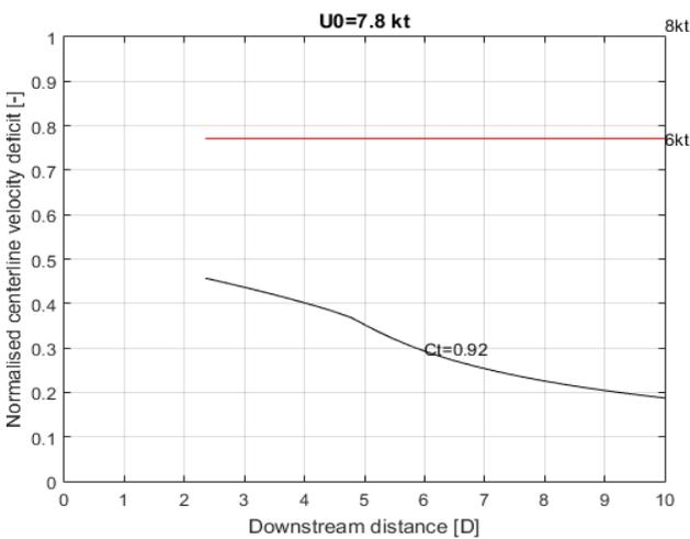
Figure 1 Normalized velocity deficit for  $U_0=4\text{m/s}$  and  $C_t=0.92$ .
