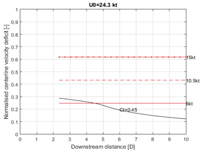
Figure 2 Normalized velocity deficit for  $U_0=12.5\text{m/s}$  and  $C_t=0.45$ .
