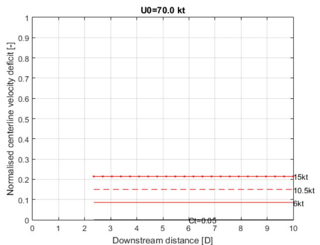
Figure 4 Normalized velocity deficit for  $U_0=36\text{m/s}$  and  $C_t=0.05$ .
