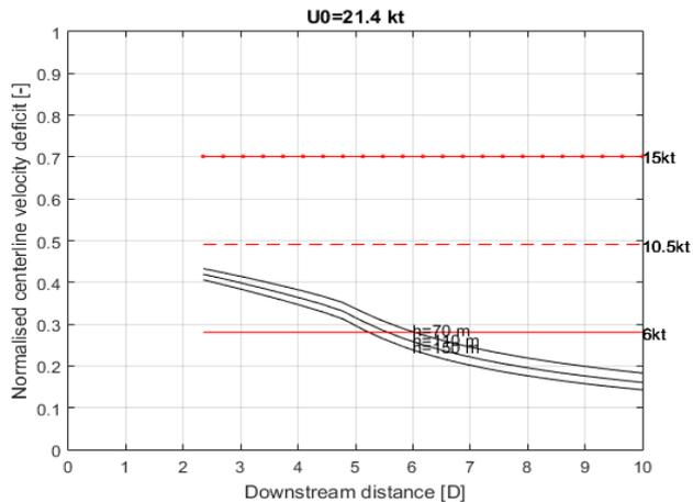
Figure 7 Normalised velocity deficit for  $U_0 = 11\text{m/s}$  and  $C_t = 0.67$ , for axis height of 70m (top), 110 and 150m (bottom)
