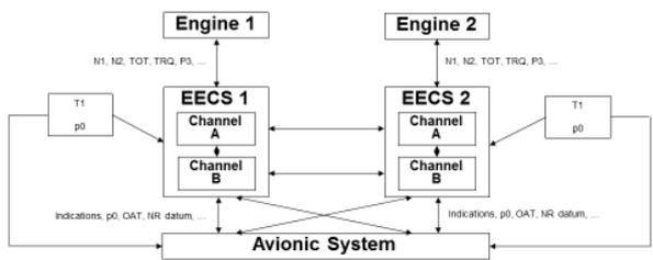
**Figure 5: EECS Block Diagram**
