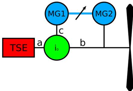
Figure 3: Input Split drivetrain
