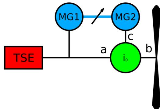
Figure 2: Output Split drivetrain
