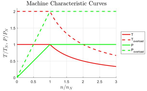
Figure 8: Characteristic curves of variator machines
