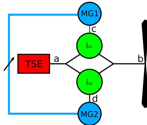
Figure 4: Compound Split drivetrain
