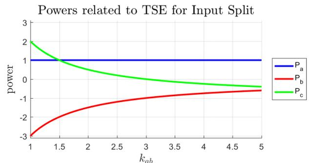
Figure 6: Shaft powers for Input Split architecture
