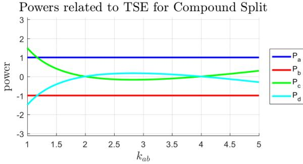
Figure 7: Shaft powers for Compound Split architecture
