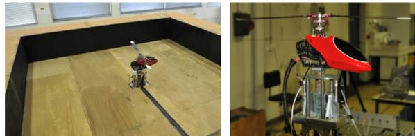
Figure 1: ONERA experiment: helicopter mounted in a square-shaped box representing a closed courtyard
