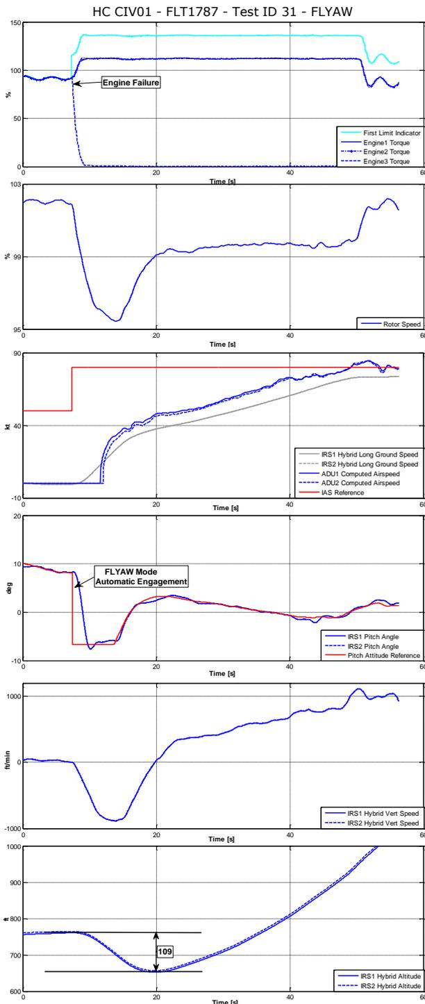
Figure 8 – FLYAW Mode Flight Test Results
