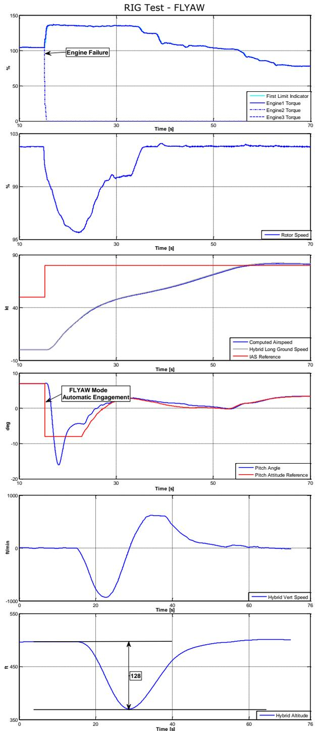
Figure 7 – FLYAW Mode HIL Rig Test Results
