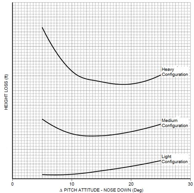
Figure 5 - Height Loss vs Initial Pitch Attitude Delta
