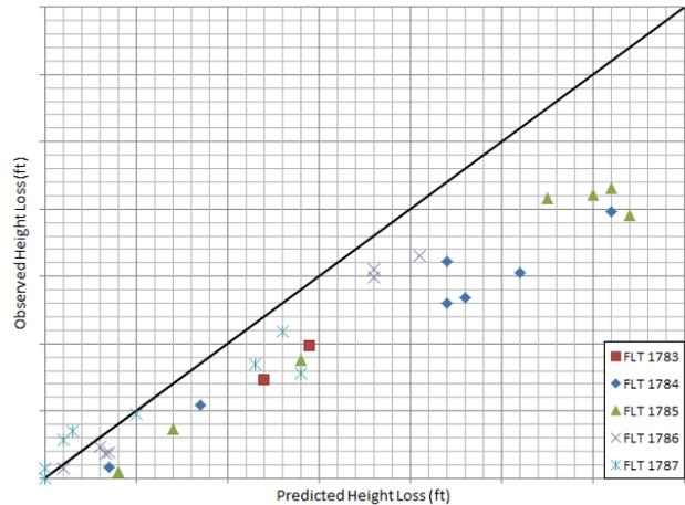
Figure 9 - Flight Test Activity Observed Height Loss Vs Predicted Height Loss
