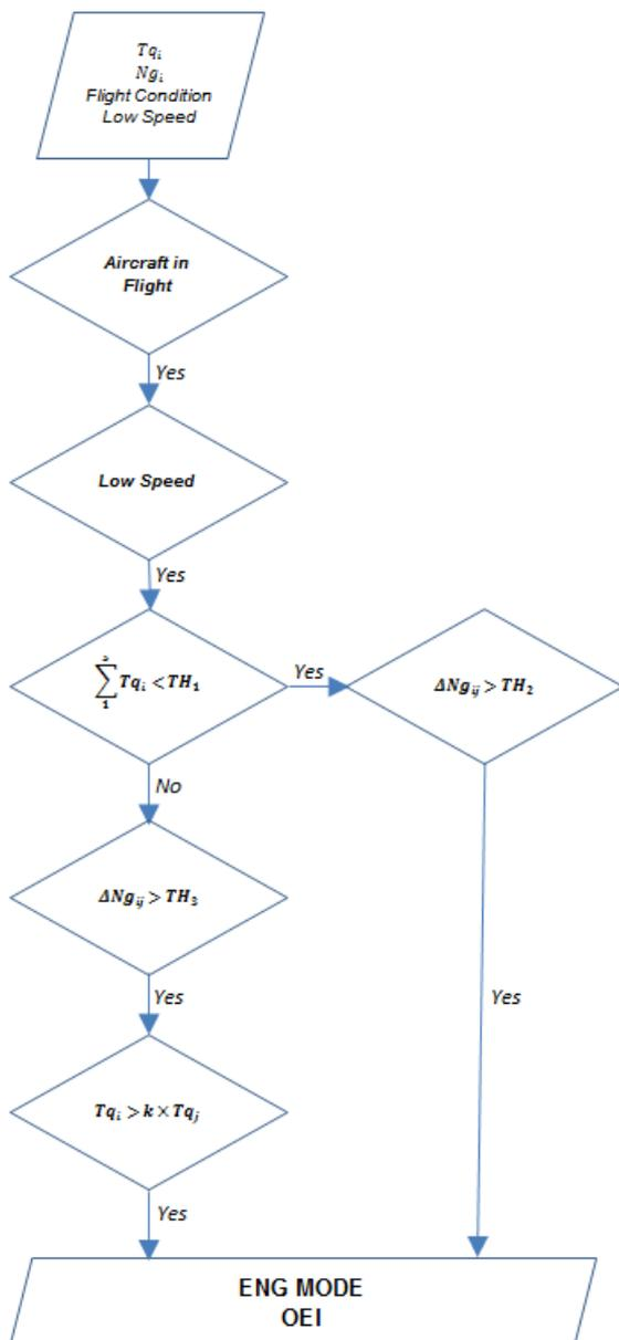
Figure 4 – AFCS Engine OEI Algorithm
