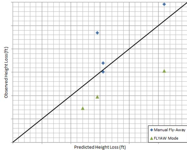
Figure 10 - Comparison between Manual and Automatic Fly-Aways
