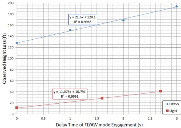
**Figure 12 - Impact of Engine Failure Detection Delay Time on Height Loss**
