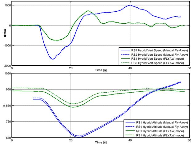
Figure 11 – Example Comparison between Manual and Automatic Fly-Away
