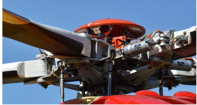
Figure 7: Main rotor head of the instrumented AW139 used for the rotor state measurement system flight demonstration.
