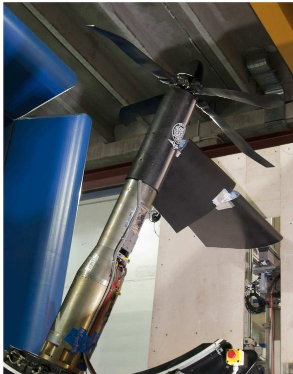
Figure 2: The tiltwing half-span model in the open test section of the Politecnico di Milano Large Wind Tunnel.
