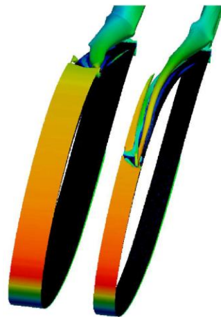
Figure 5: Comparison of the vortex generators and the trailing vortex before (left) and after (right) the optimisation, based on the NACA64(4)-421 aerofoil, performed by the University of Bristol [13].
