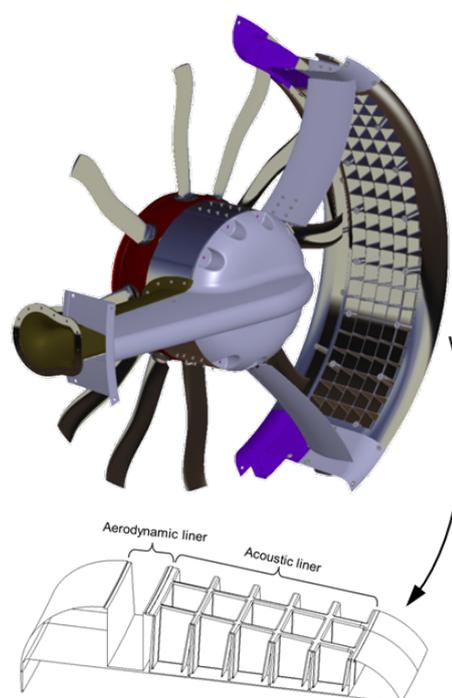
**Figure 20: Advanced Fenestron® lining concept**
