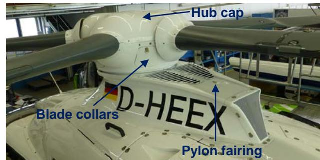
**Figure 7: Detail of the semi water-tight full faring about the 5-bladed BMR of the BD**
