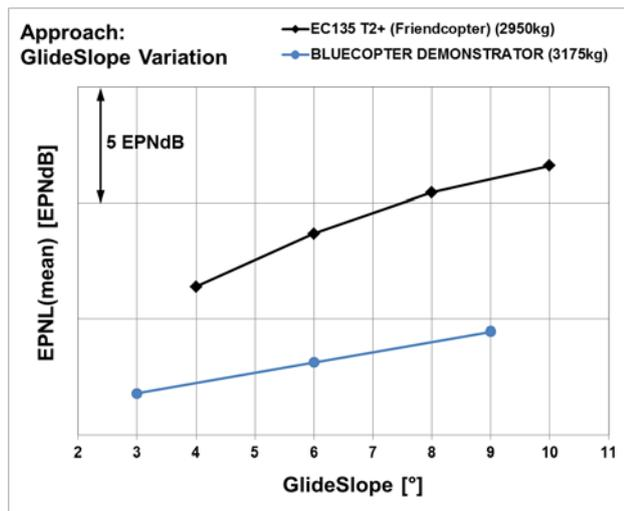
Figure 18: Glide slope variation at  $V_y$  with a fixed height above the microphone
