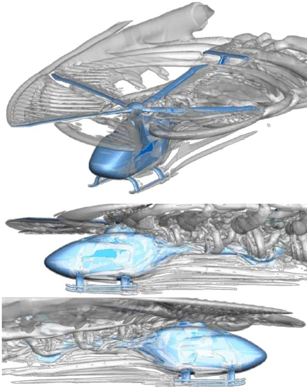
**Figure 10: Coupled CFD-CSM simulation in level flight @ 130kts: wake system visualized by the  $\lambda_2$  criterion**
