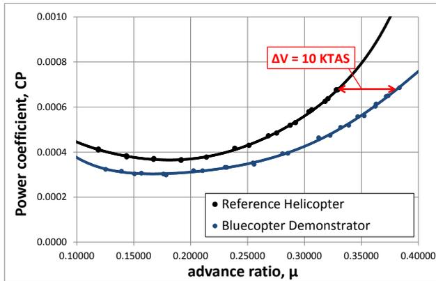
**Figure 14: Comparison of power required in forward flight between reference helicopter and Bluecopter demonstrator**
