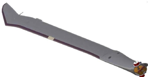
**Figure 1: BlueEdge™ style main rotor blade**
