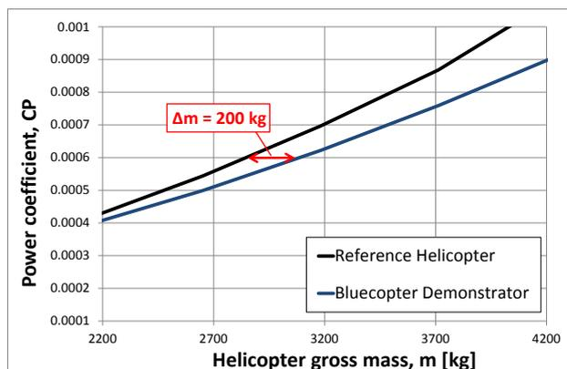
**Figure 13: Power required of the helicopter as a function of reduced gross mass  $m$  in hover out of ground effect**
