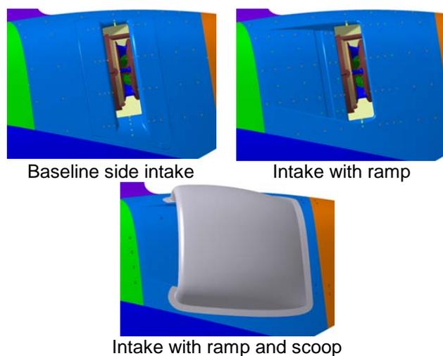
**Figure 21: Side intake variants for the BD**
