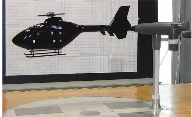
**Figure 6: Serial EC135 wind tunnel model (scale 1:7) in the TUM-AER facility A**
