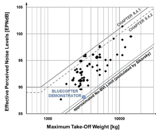
Figure 19: Noise certification approach levels vs. maximum take-off weight compared for ICAO Annex 16, Chapter 8 helicopters
