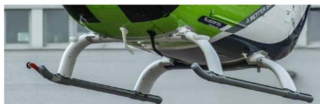
**Figure 4: Detail of the landing skid fairings on the BD**
