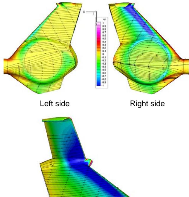
**Figure 9: Pressure coefficient with superimposed friction lines on the BD tail unit (level flight 130kts)**
