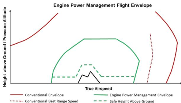
**Figure 12: Flight envelope applicable to engine power management**
