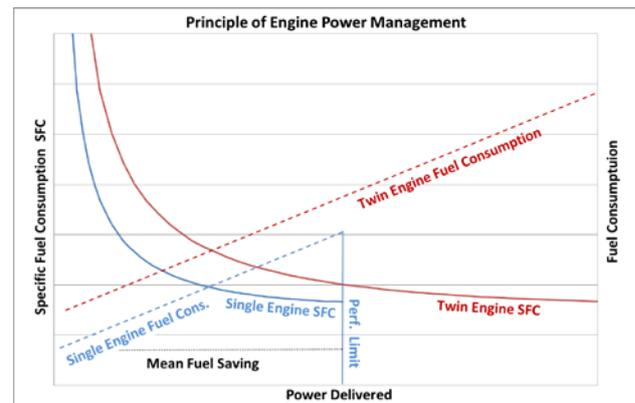
**Figure 11: Characteristic engine efficiency behavior and effect on power management**
