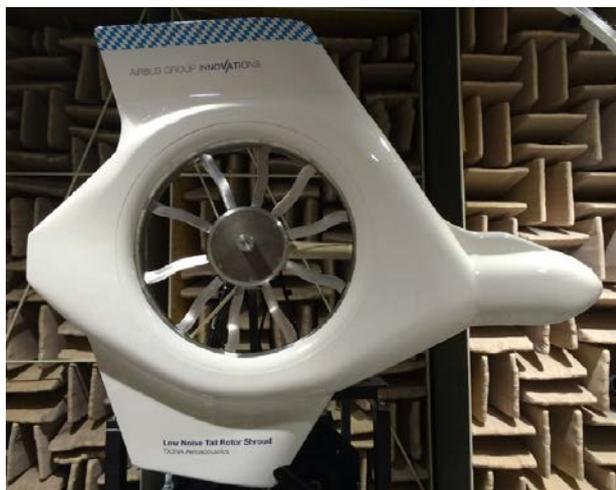
**Figure 3: Fenestron® test bench @ Airbus Group Innovations (Ottobrunn)**
