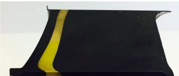
Figure 13: Tube-Form Cross-Section with Embedded Marker Layer
