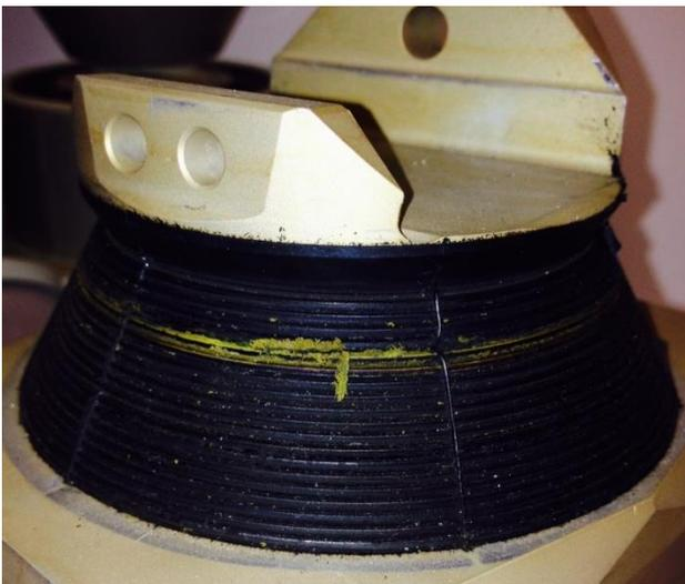
Figure 8: Example of Colored Crumbing at the Surface
