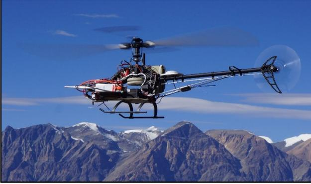
Fig.8: Helicopter (GW about 5kg) modified for high altitude measurements, HOGE at 5170m MSL
