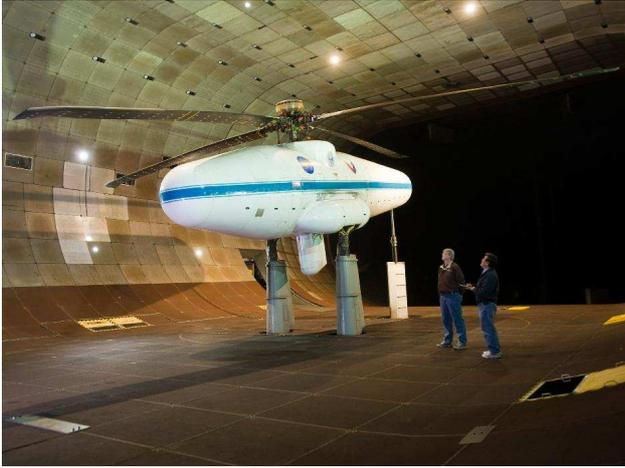
(a) Full-scale UH-60A rotor installed on the Large Rotor Test Apparatus in the NFAC 40- by 80- ft wind tunnel.
