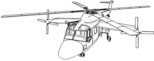
**Fig. 1. Sketch of the Hybrid Compound Helicopter (HCH) Configuration.**
