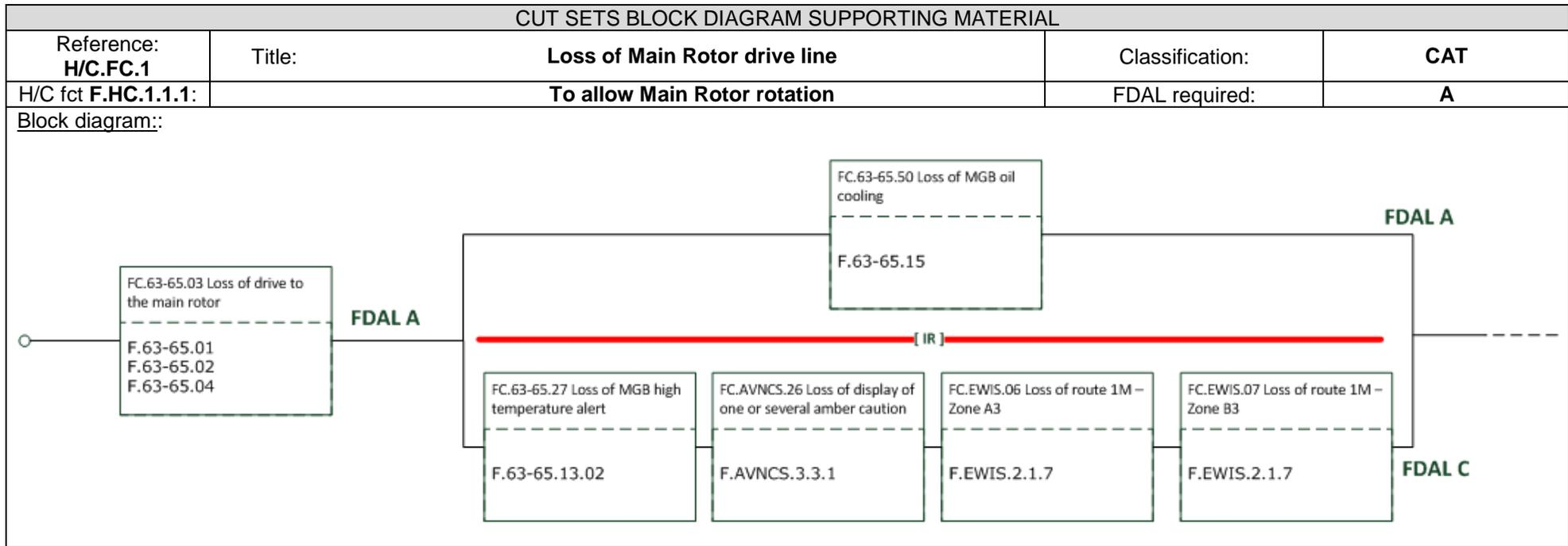
Figure 12: Example of Cut-sets diagram
