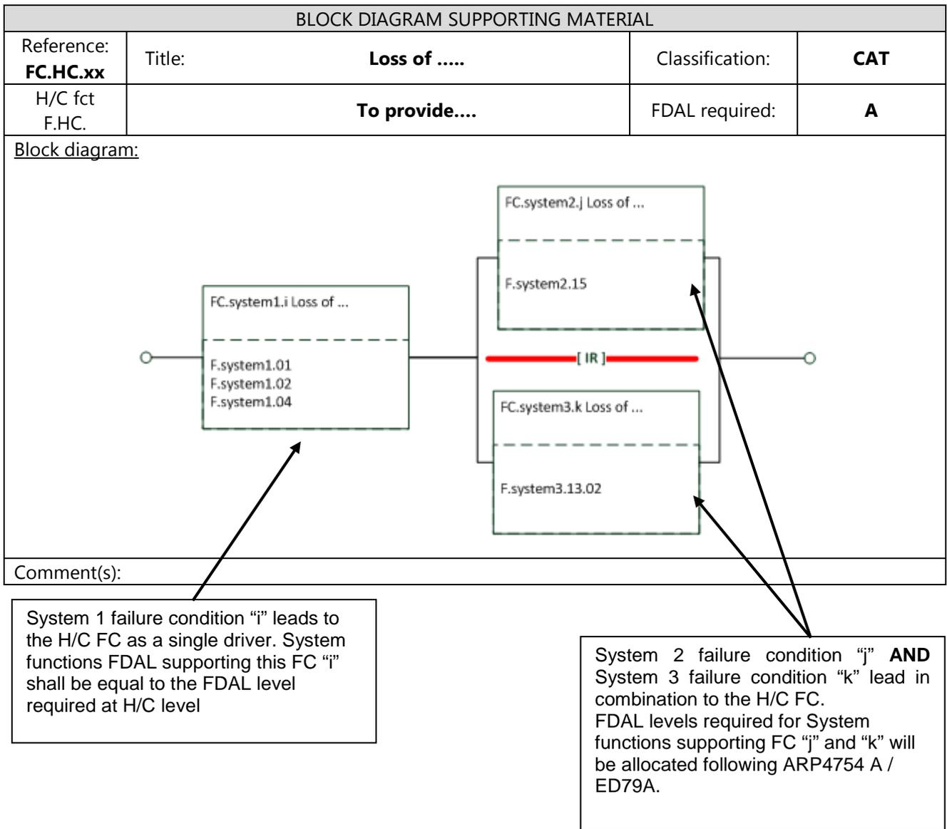
Figure 11: chart of Cut-sets diagram
