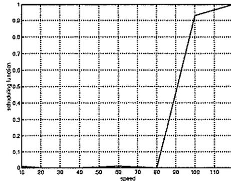
Figure 4: Scheduling function vs forward speed
