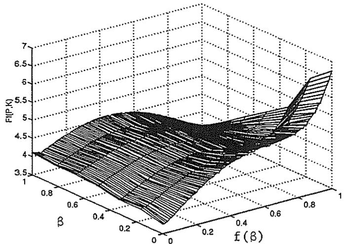
Figure 3: Cost function across the operating envelope.  $f(\beta)$  - controller scheduling function,  $\beta$  - normalised forward speed,  $\mathcal{F}(P, K)$  - cost function
