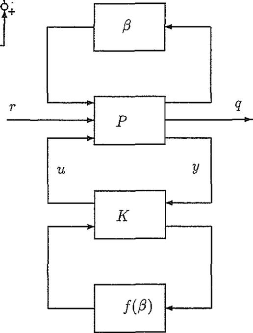
Figure 2: Linear Fractional Transformation of the gain scheduled system
