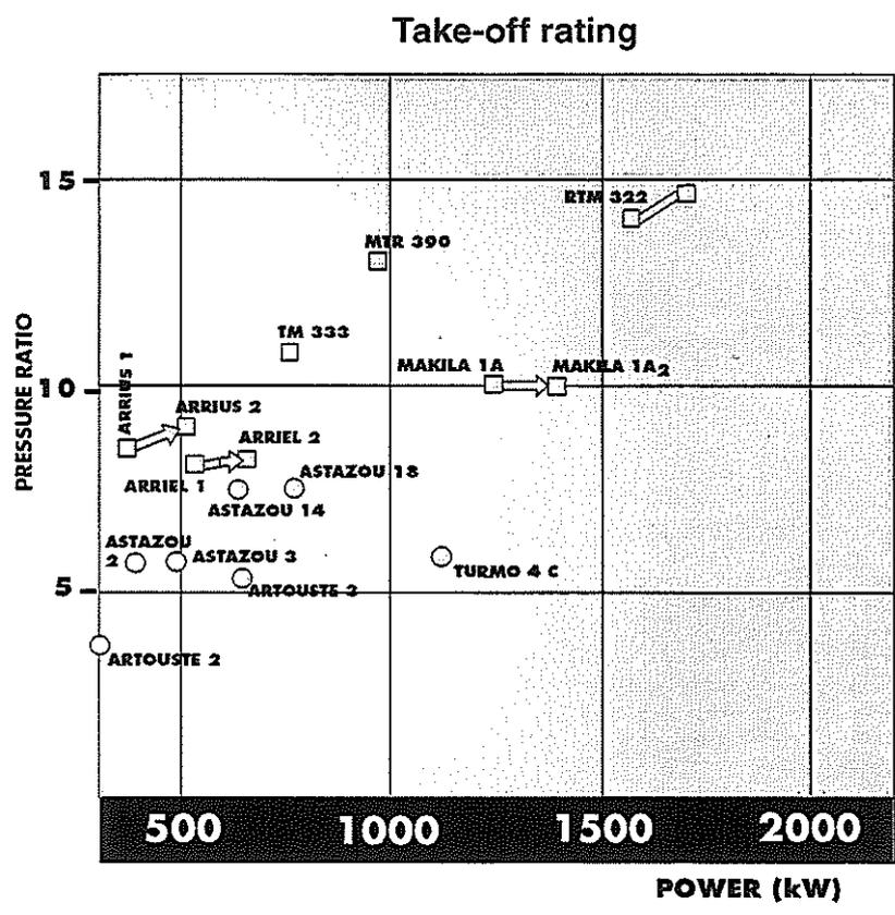
FIG. 6 Pressure ratio increase
