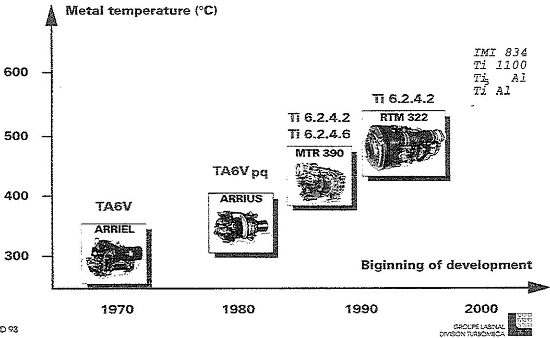
**FIG. 15** Titanium alloys applied to centrifugal impellers
