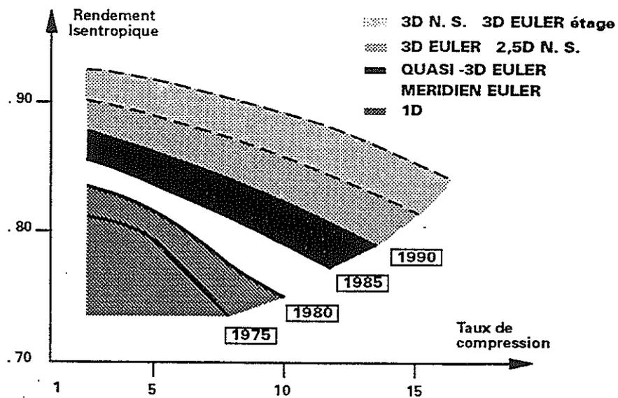
**FIG. 13** Single stage centrifugal compressor
