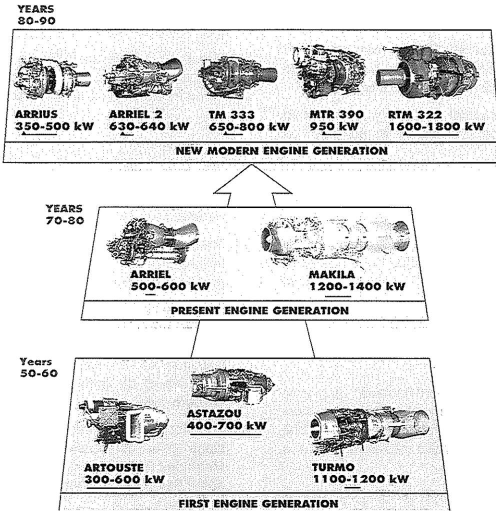
**FIG. 1** Turbomeca experience in the field of helicopter power plants
