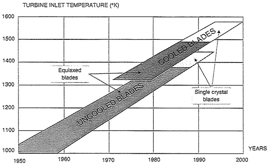
**FIG. 19 Turbine material evolution**
