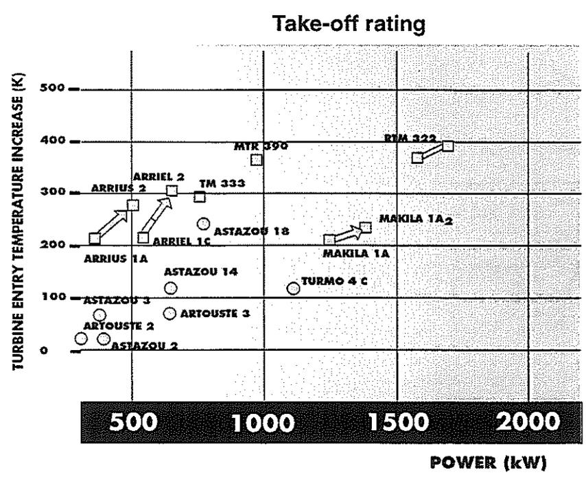
FIG. 7 Turbine entry temperature increase
