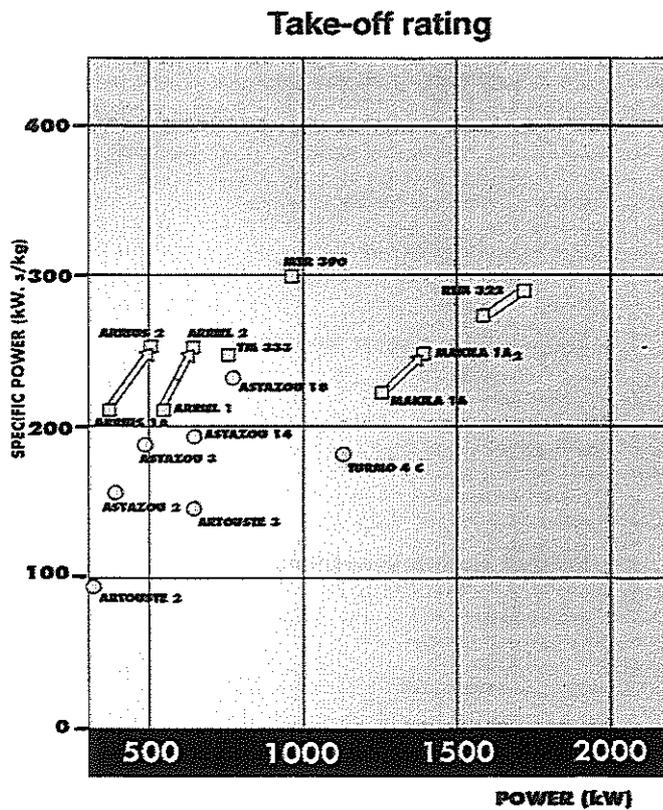
FIG. 3 Power to weight ratio evolution
