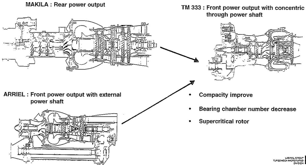
FIG. 10 Architecture evolution : Power shaft
