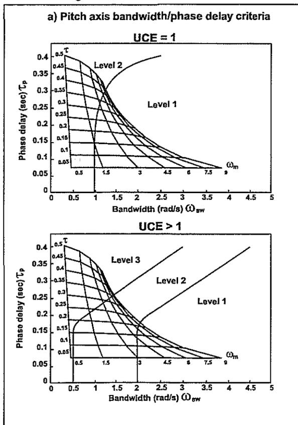
A further point to note is that test cases are only nominally labelled as either Level 1, 2 or 3, which signifies that the individual criteria for the roll and pitch axes were set at that level. This is because the ADS criteria only purport to predict that a configuration will have overall Level 1 handling qualities if all of the Level 1 criteria and conditions are met; failure to meet one or more of these can have a synergistic effect that may cause handling
