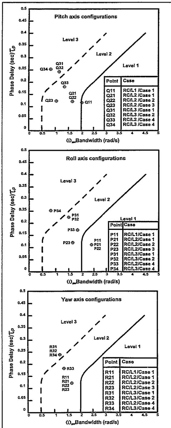
Fig 4 ACAH configurations versus attitude bandwidth criteria for UCE>1
