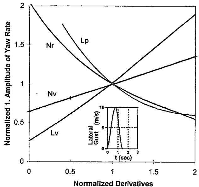
Fig. 25 Influence of characteristic derivatives on gust response for yaw axis (90 kts MCP)
