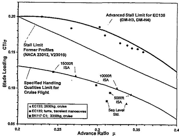
Fig. 22 Operational limits in the blade loading diagram
