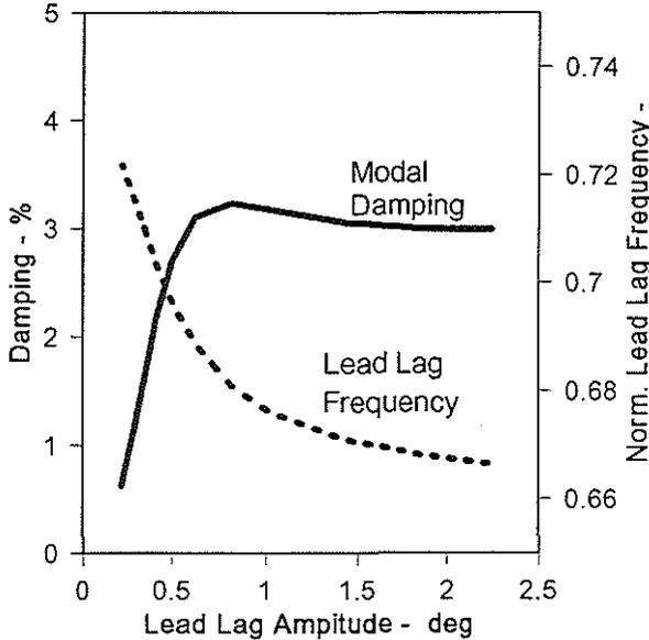
Fig. 8 Modal damping and lead lag frequency versus lead lag amplitude
