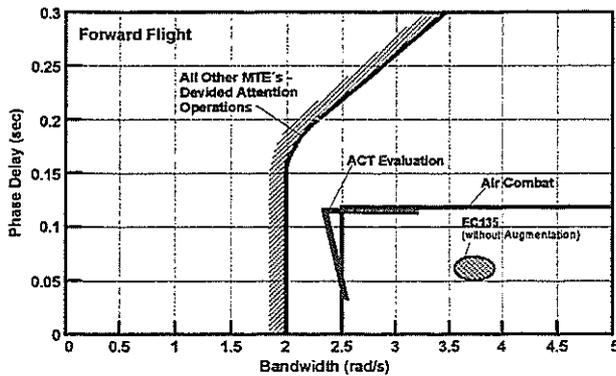
Fig. 24 Phase delay vs. bandwidth for the roll axis (small amplitude criteria of ADS-33D)
