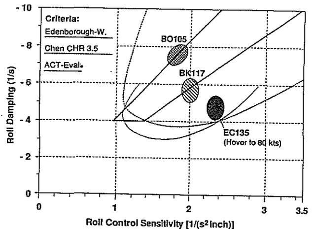
Fig. 23 Controllability chart for the roll axis
