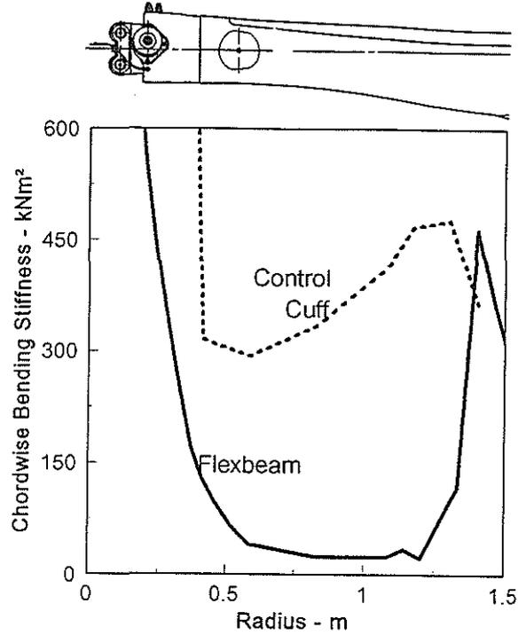
Fig. 6 Chordwise bending distribution of the Flexbeam and the control cuff
