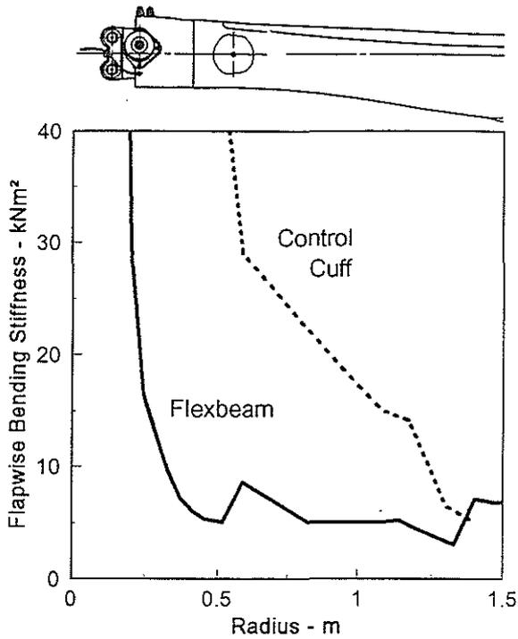
Fig. 4 Flap bending distribution of the flexbeam
