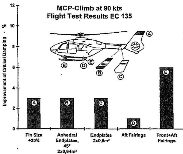
Fig. 19 Aerodynamic measures to improve critical dutch roll damping
