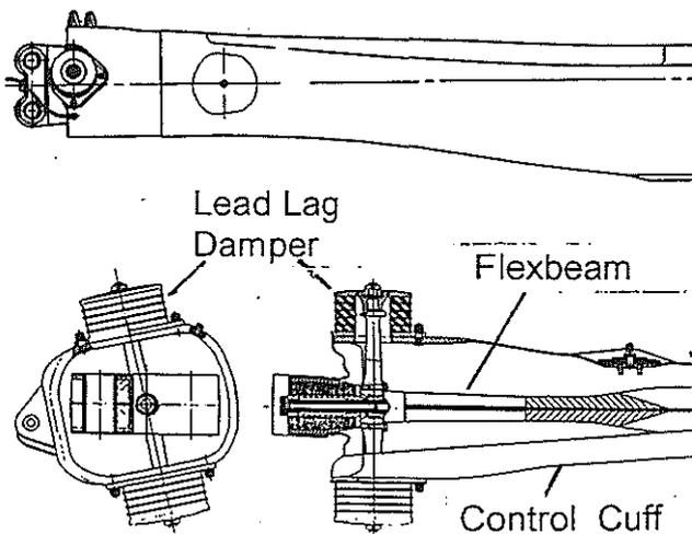
Fig. 5 Design of flexbeam and control cuff
