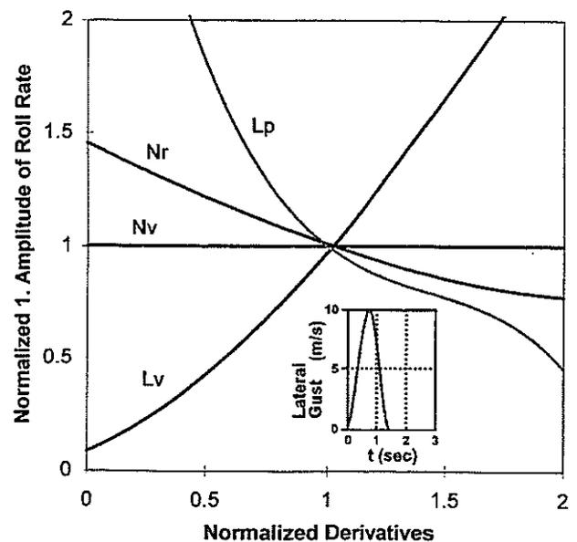
Fig. 26 Influence of characteristic derivatives on gust response for roll axis (90 kts MCP)
