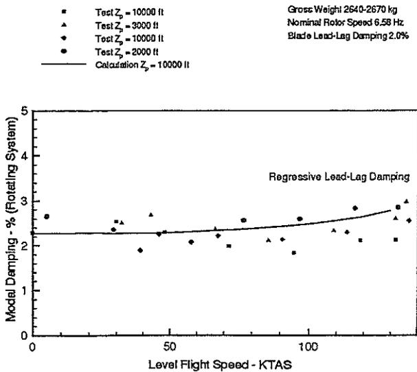
Fig. 12 Air resonance stability
