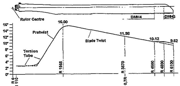
Fig. 16 Twist distribution along blade span
