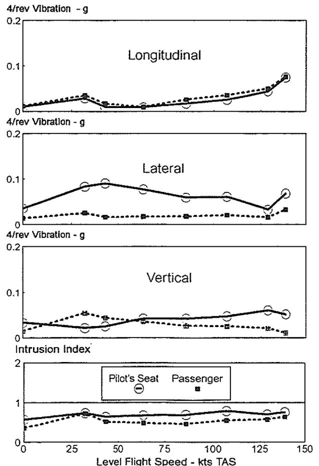
Fig. 13 Cabin vibrations during level flight
