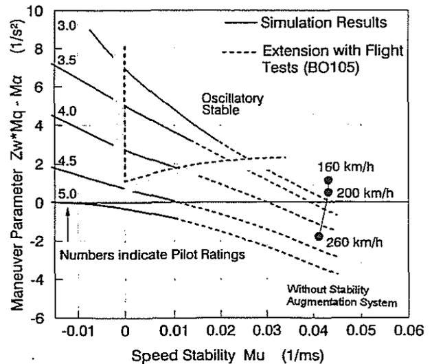
Fig. 20 Relationship between longitudinal derivatives and pilot ratings
