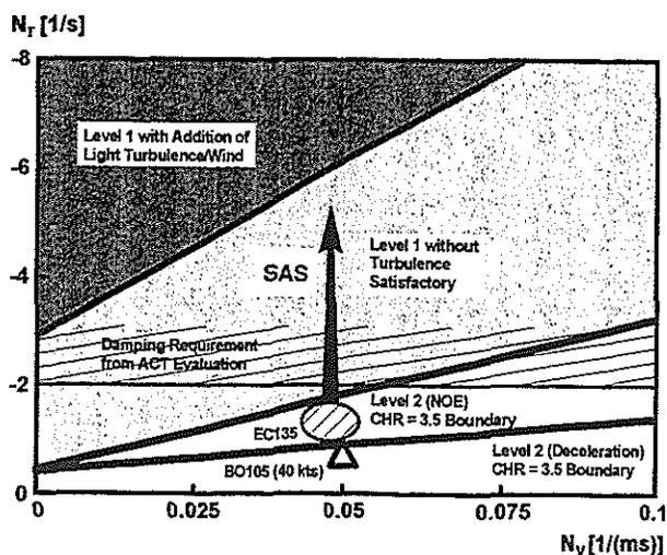
Fig. 27 Yaw damping requirements in gusty flight conditions (from [19])
