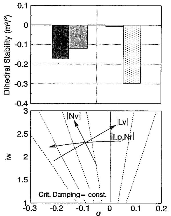
Fig. 18 Significant derivatives for dutch roll and their influence on critical dutch roll damping
