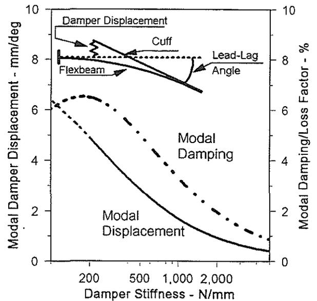
Fig. 7 Chordwise kinematics determines displacement and damping of the damper
