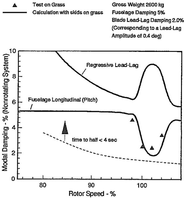
Fig. 11 Ground resonance stability
