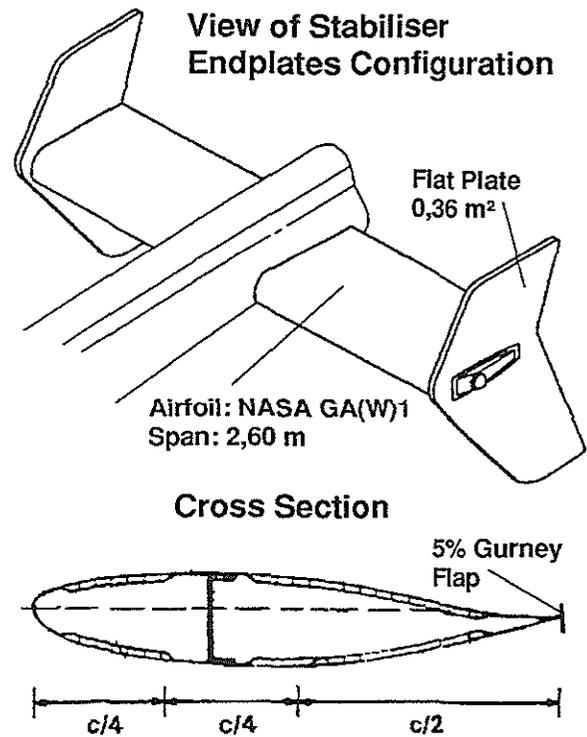
Fig. 21 Configuration of horizontal stabiliser with Gurney flaps
