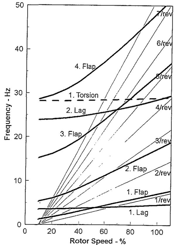
Fig. 10 Tuning of the higher blade modes
