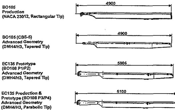
Fig. 14 Advanced blade planforms developed for BO105 CBS-5 and EC135
