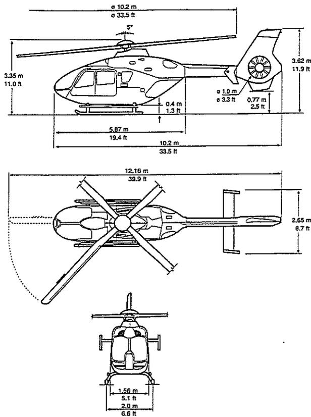
Fig. 2 General dimensions of EC135
