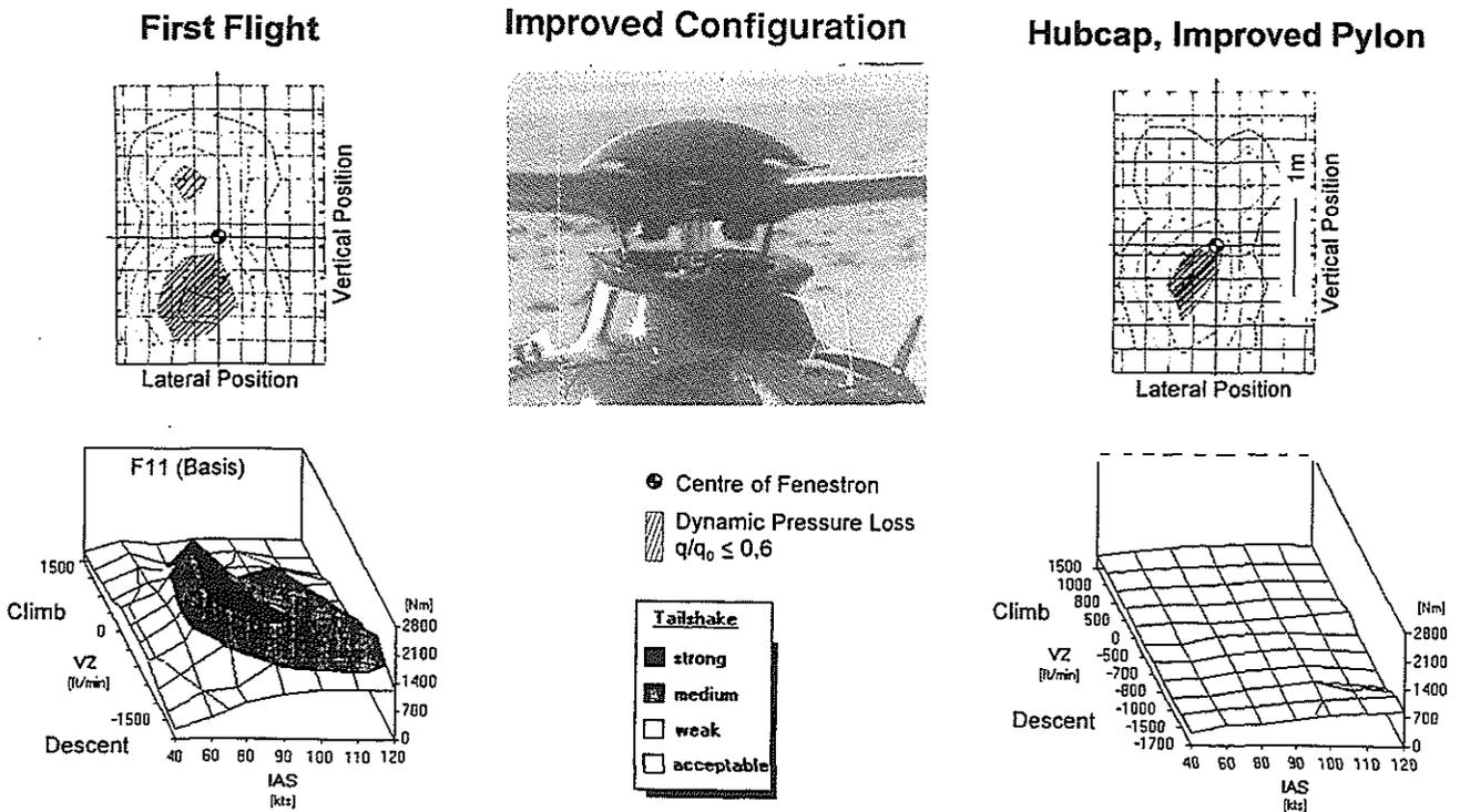
Fig. 17 Reduction of tail shake with hub cap and pylon
