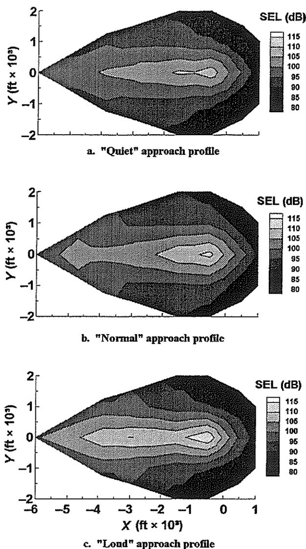
Fig. 6. Measured noise footprints. (Courtesy of NASA)
