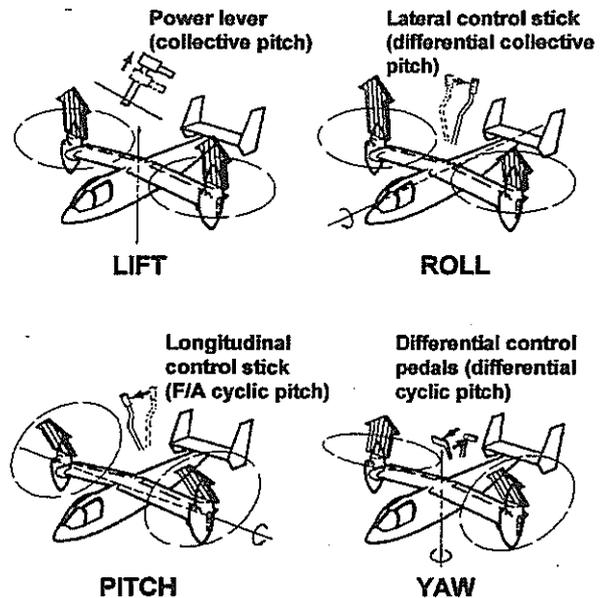
Fig. 2. Flight control functions in helicopter mode.
