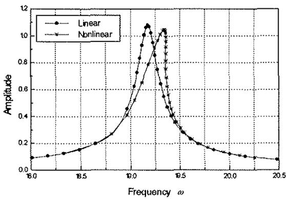
Fig. 3 hard spring characteristic of the structure
