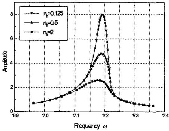
Fig. 1 effect of different damp ( $\eta_r=0.3N$ )
