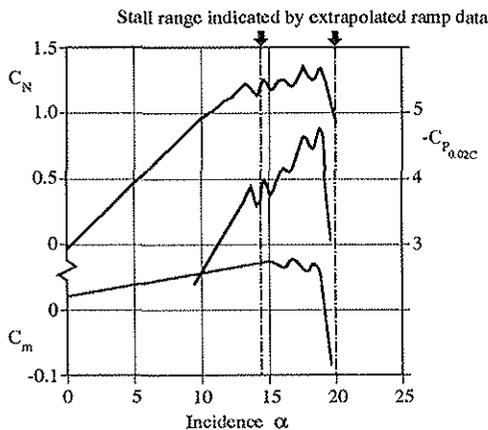
Fig 13 Quasi-Steady Normal Force and Pitching Moment Coefficients for RAE 9651 at  $M = 0.3$
