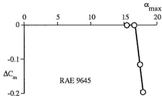
Fig 4 Pitching Moment Deviation in Oscillatory Pitch Cycles
