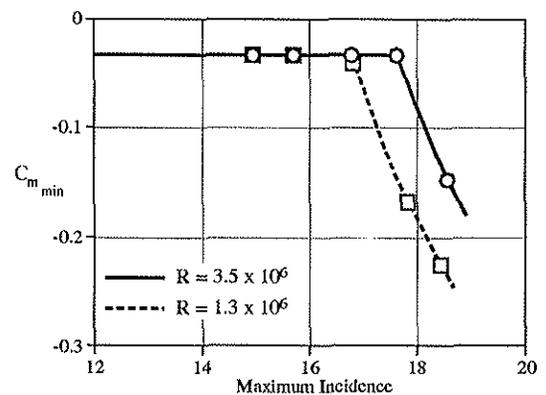
Fig 14 Effect of Reynolds Number on "Critical" Incidence for RAE9646 at M = 0.3
