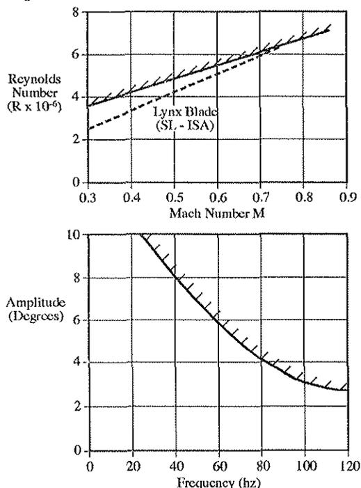
Fig 2 Operating Range for Dynamic Test Rig
