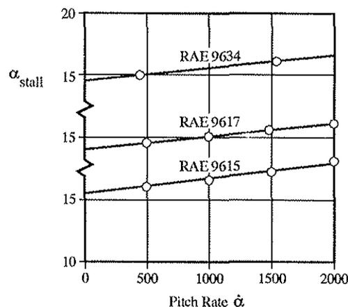
Fig 7 Variation of Stall Incidence with Pitch Rate
