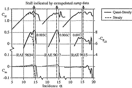
Fig 8 Quasi-Steady Test Data for Thin Aerofoils at  $M = 0.3$
