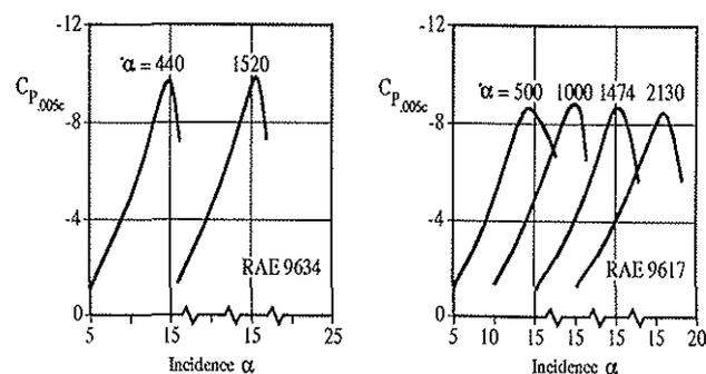
Fig 6 Variation of Leading-Edge Suction Peak with Incidence for Various Pitch Rates
