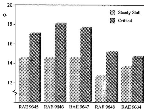
Fig 5 Comparison of Steady Stall Incidence with "Critical" Incidence, at M = 0.3
