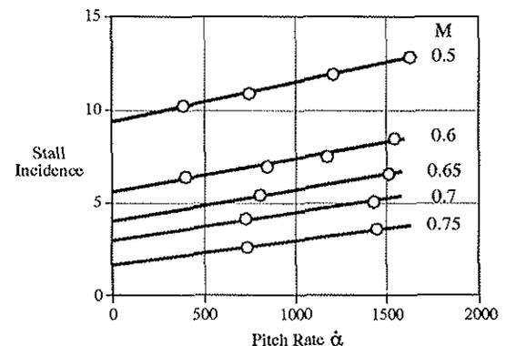
Fig 15 Variation of Stall Incidence with Pitch Rate for RAE 9646 at A Range of Mach Numbers
