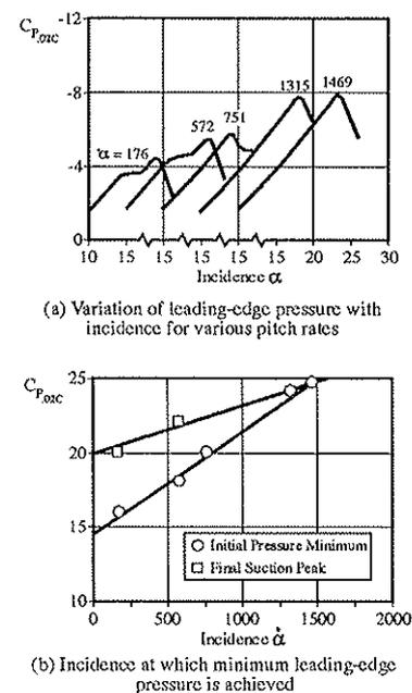
Fig 12 Ramp Test Characteristics for RAE 9651
