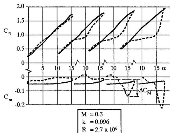
Fig 3 Variation of Normal Force and Pitching-Moment Coefficient with Incidence During A Series of Pitch Cycles for RAE 9645
