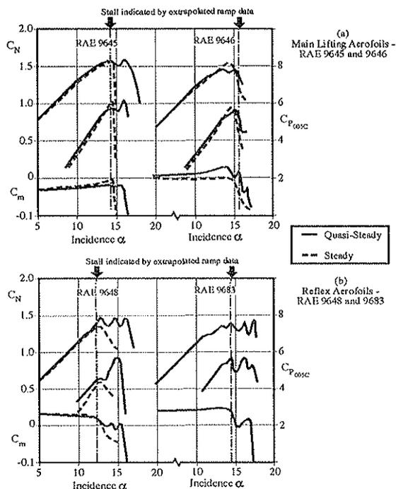
Fig 11 Quasi-Steady Characteristics at  $M = 0.3$  with Stall Incidence from Extrapolated Ramp Tests
