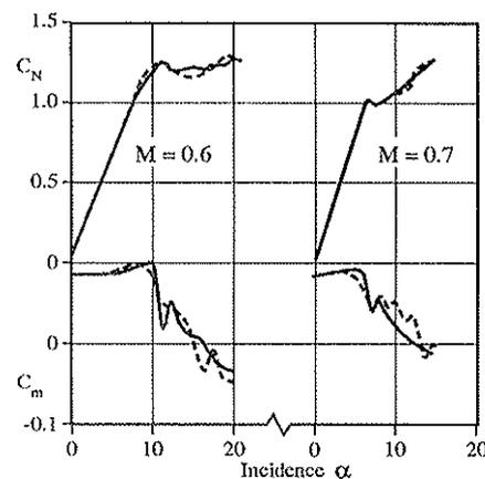
**Fig 17 Modelled and Measured Variation of  $C_N$  and  $C_m$  with Incidence for RAE9634 at Steady Pitch Rate**
