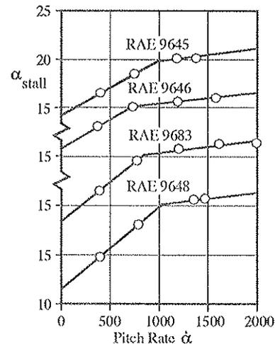
Fig 10 Variation of Stall Incidence with Pitch Rate
