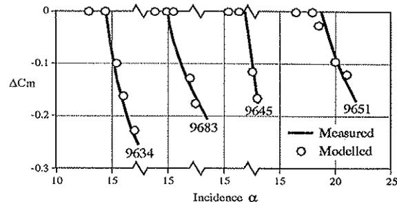
**Fig 16 Modelled and Measured Pitching Moment Deviation in Oscillatory Cycles**
