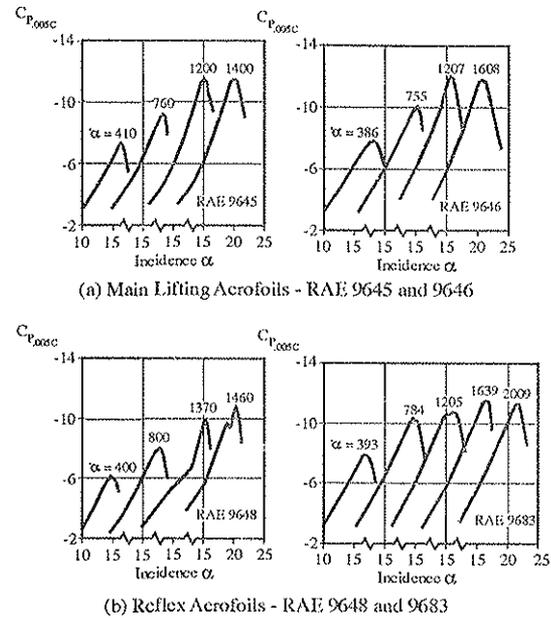
Fig 9 Variation of Leading-Edge Suction Peak with Incidence for Various Pitch Rates
