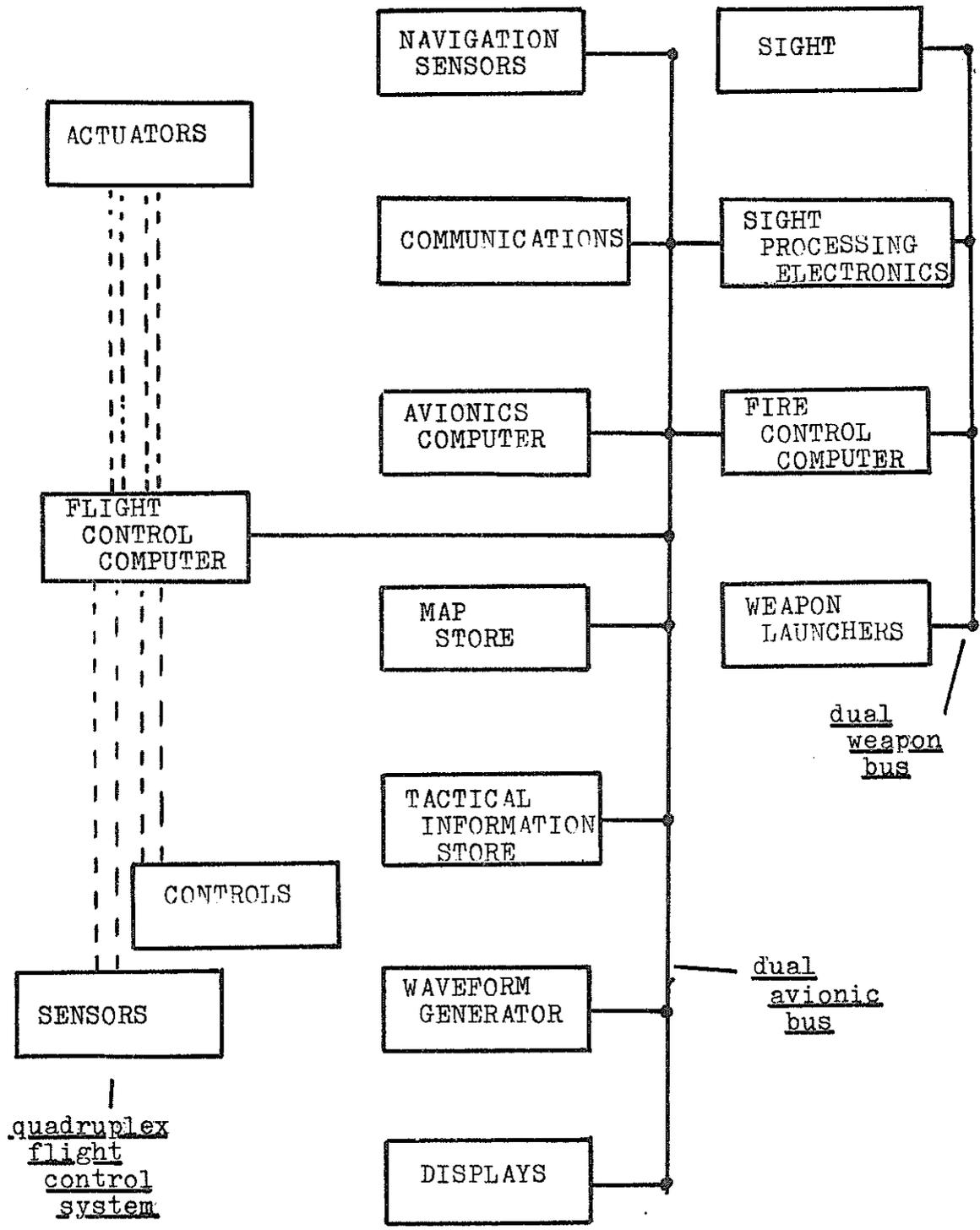
FIGURE 2 Schematic outline of a fully integrated helicopter flight control, avionic, and weapons system.
