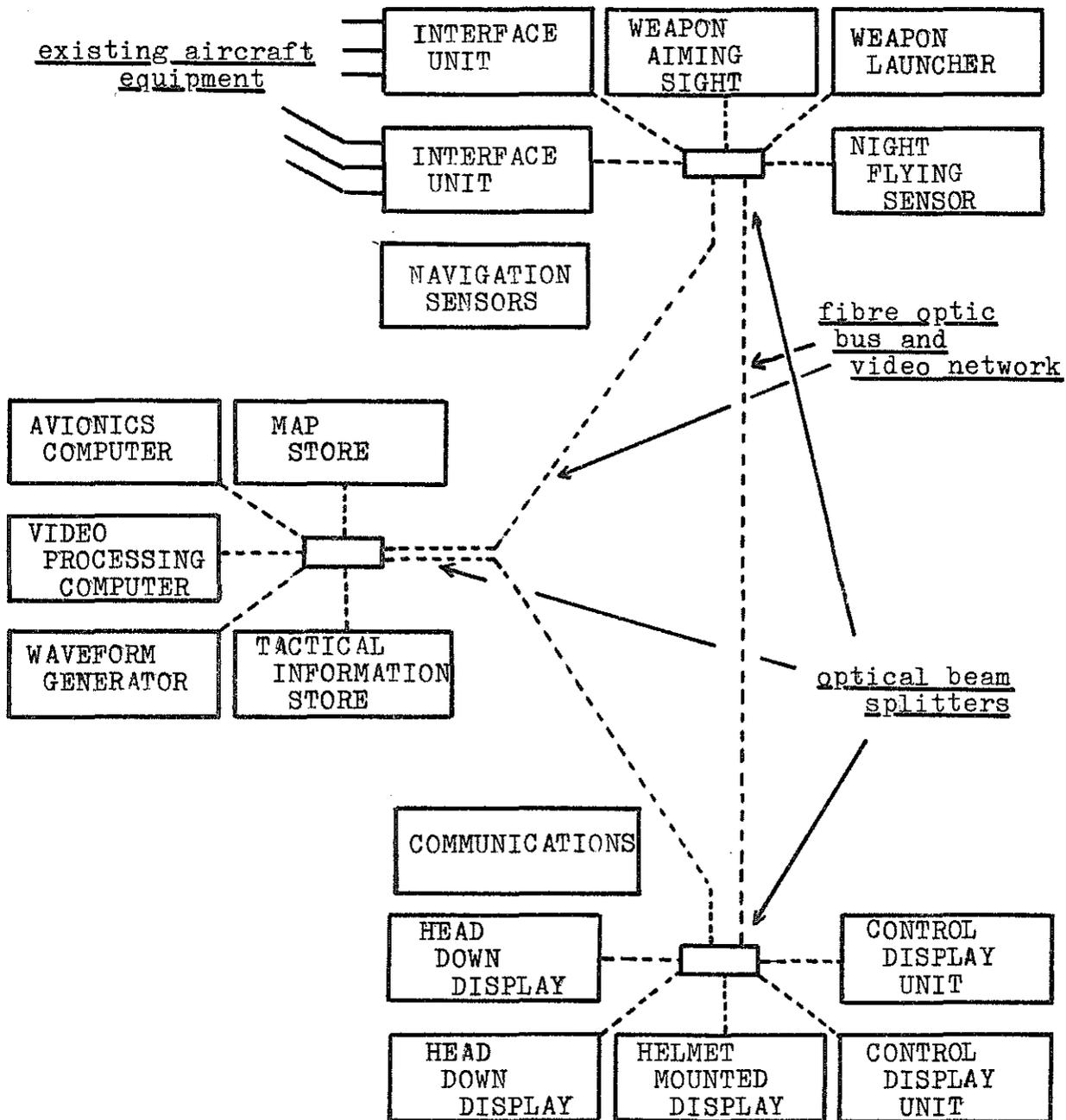
FIGURE 1 Schematic outline of the Integrated Avionics and Weapon System to be installed in a Lynx Helicopter at Farnborough.
