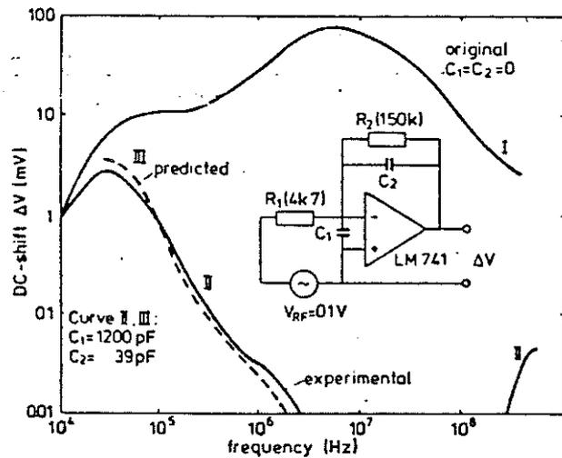
FIG. 6 DC shift as a function of frequency
