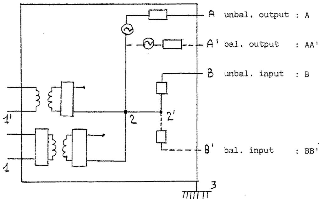
FIG. 1 Grounding diagram
